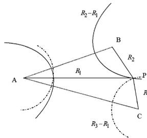
**Figure 4<sup>[7]</sup> Positioning based on TDOA Measurements**
