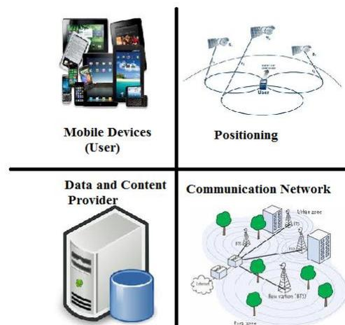
**Figure 1: The Basic Components of LBS.**
