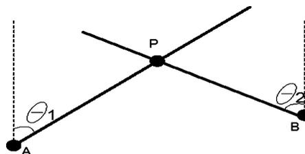
Figure 2<sup>[7]</sup>: Positioning based AOA measurement.
