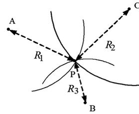
**Figure 3<sup>[7]</sup>: Positioning based on TOA measurements**
