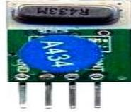
**Figure 3:** RF Transmitter
