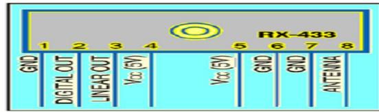
Fig3: PIN CONFIGURATION OF RF RECIEVER MODULE
