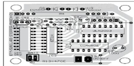
Fig. 7: Component layout for the PCB shown in Fig. 8
