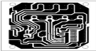
Fig. 4: Actual-size, single-side PCB for the transmitter circuit
