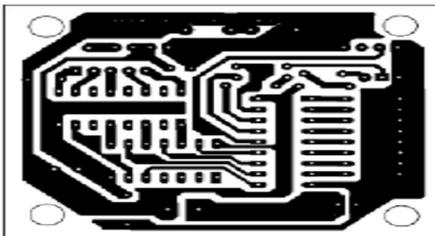
Fig. 6: Actual-size, single-side PCB for the receiver-cum decoder circuit.
