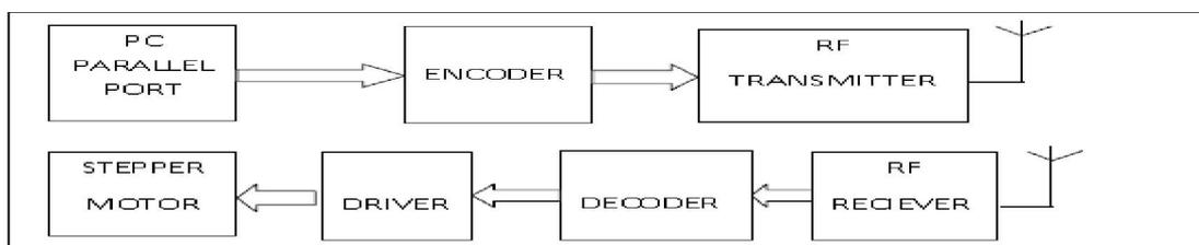
Fig1: Block diagram for PC based wireless control of stepper motor
