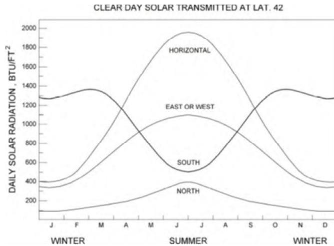
**Figure 7.** On June 21, windows orientations receive the maximum solar radiation in the summer, except skylights on the south orientation, which receive four times more than south-oriented windows (by Balcomb, 1987)
