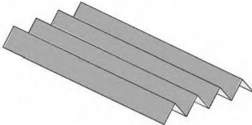
**Figure 10.** Longitudinal folding surface (by Hanaor & Levy, 2001)
