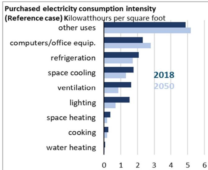
**Figure 4.** Electricity consumption by building component (U.S. EIA)
