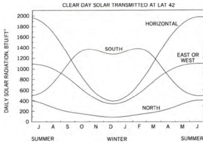
**Figure 6.** On June 21 South-oriented windows maximize solar radiation in the summer and minimize it in the winter (Balcomb, 1987)
