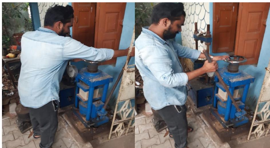
**Figure 3:** Testing Of Cubes On CTM
