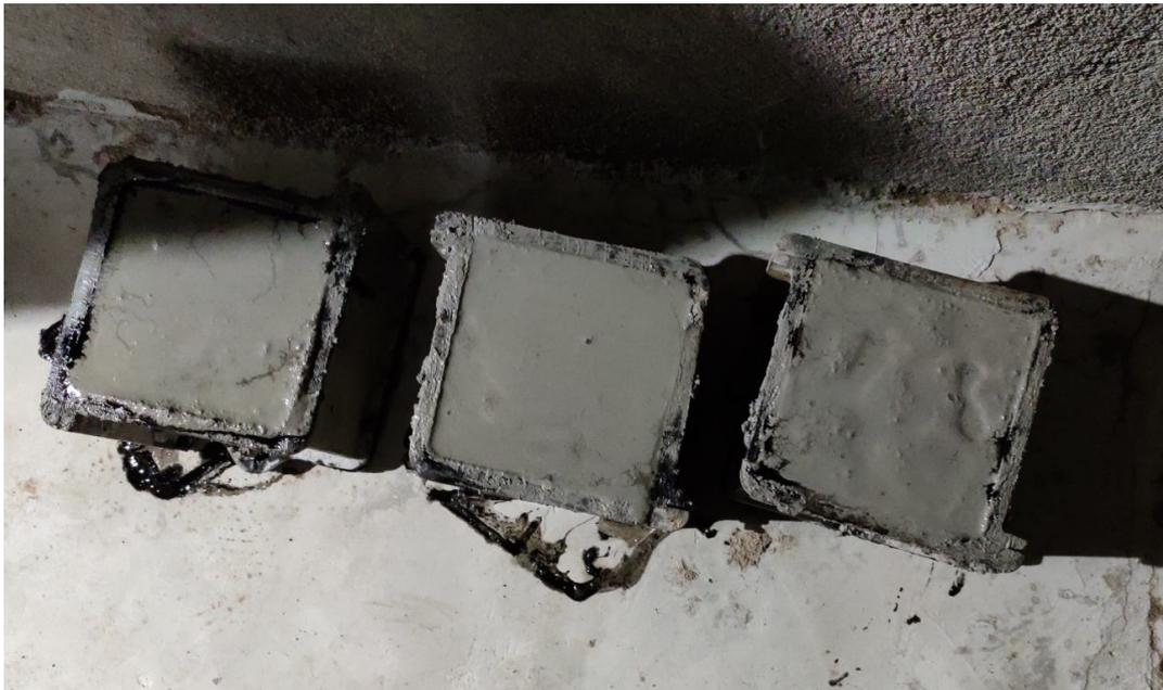
**Figure 2:** Cubes For Testing
