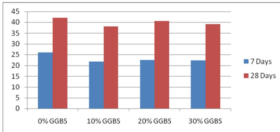
**Figure 4:** Graph of Compressive Strength At 7Days and 28Days
