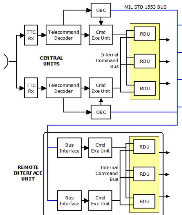
Figure 2 Block diagram of a Spacecraft Telecommand System
