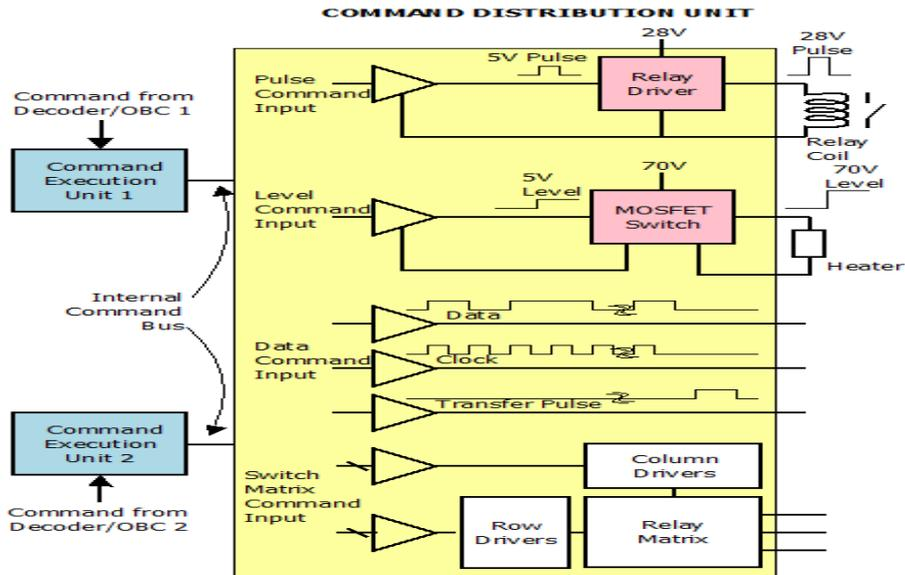
**Figure 3** Discrete Command Interfaces
