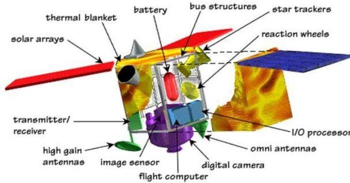
Figure 1 Subsystem in a Spacecraft
