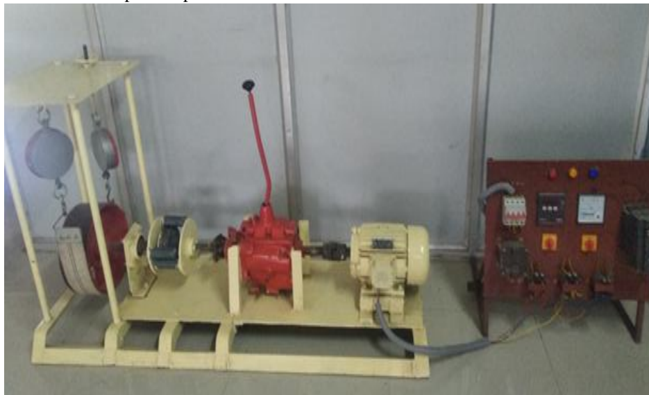
FIG.-1 Setup of Spherical Joint-lobe type flexible coupling
