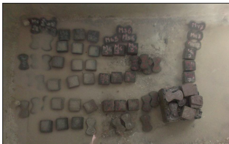
Figure 2: Test specimens for compressive strength
