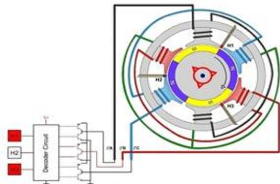
**Figure 2: BLDC Motor Winding connections**
