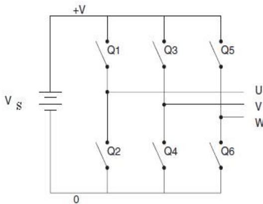
**Figure 4:** Power Circuit Diagram
