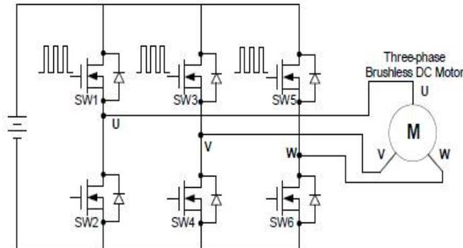
**Figure 3:** Three-phase inverter circuit powering BLDC motor
