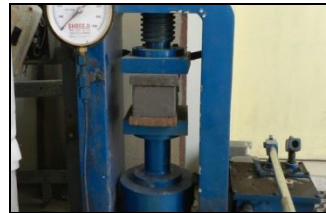
Figure 7 Compression test on cube
