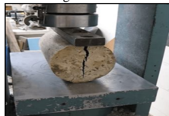
Figure 8 Split tensile strength on cylinder
