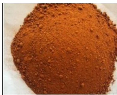
Figure 3 Crushed Spent Fire Bricks (CSFB)
