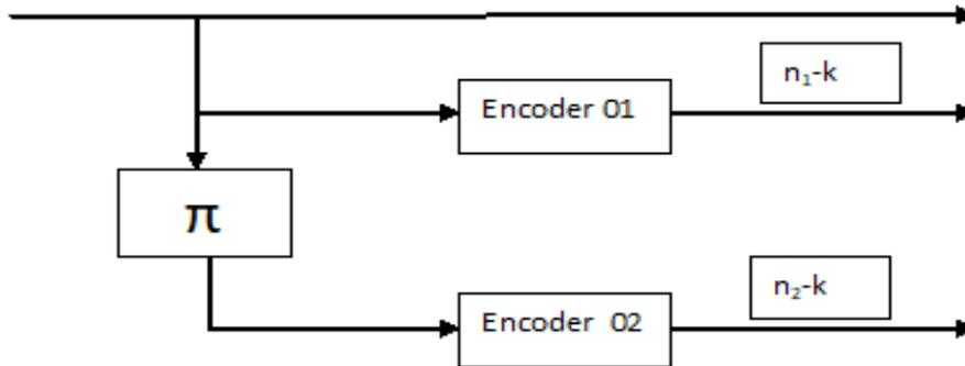
Figure 3 Parallel Interleaver
