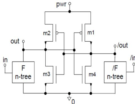
**Figure3:** 2N2N-2P energy recovery logic inverter
