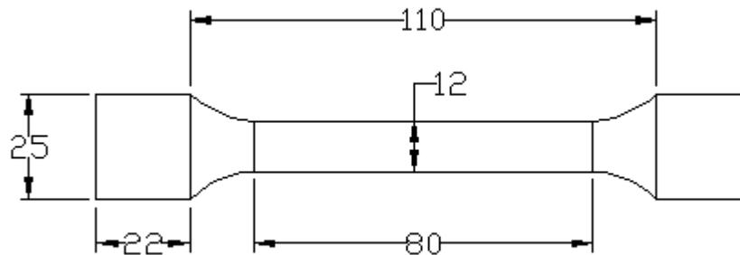
Fig.5 Design of casting of the Naval alloy
