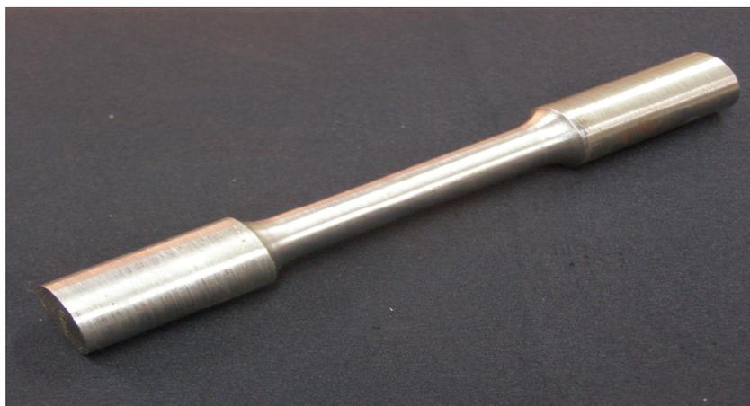
Fig.8 Finished casting of the desired alloy
