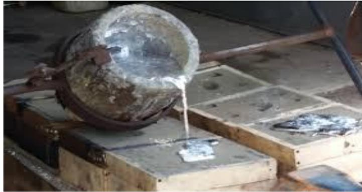
Fig.6 Molten metal pouring into the moulds
