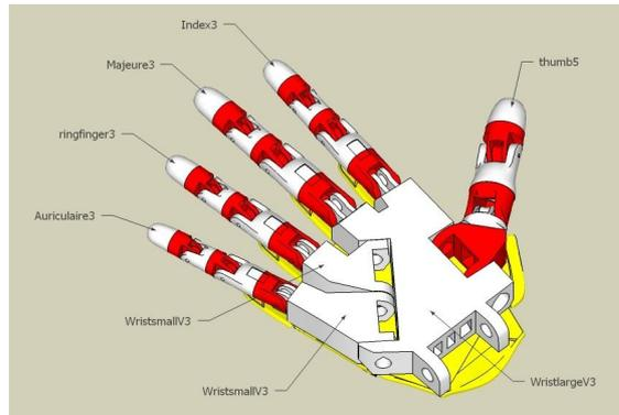
**Figure 4:** 3D CAD printable design for hand.
