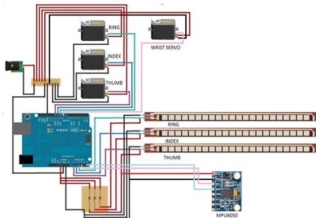
**Figure 5:** Control circuit for prosthetic hand-arm system using control glove.
