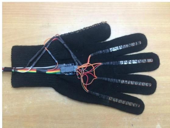
Figure 9: Control glove for prosthetic hand-arm system.
