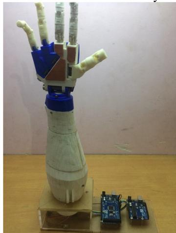
**Figure 12:** Prosthetic hand-arm system with Arduino board controller.
