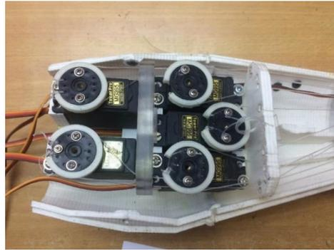
**Figure 11:** Servomotors base and nylon strings.
