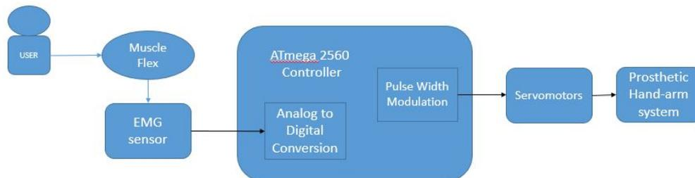
**Figure 3:** Block diagram of control flow of prosthetic hand-arm system using EMG sensor.
