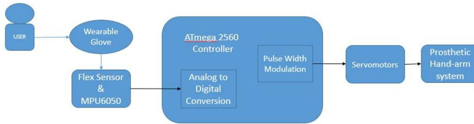
**Figure 2:** Block diagram of control flow of prosthetic hand-arm system using wearable glove.
