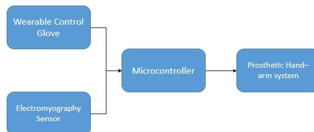
**Figure 1:** Block diagram of prosthetic hand-arm system.
