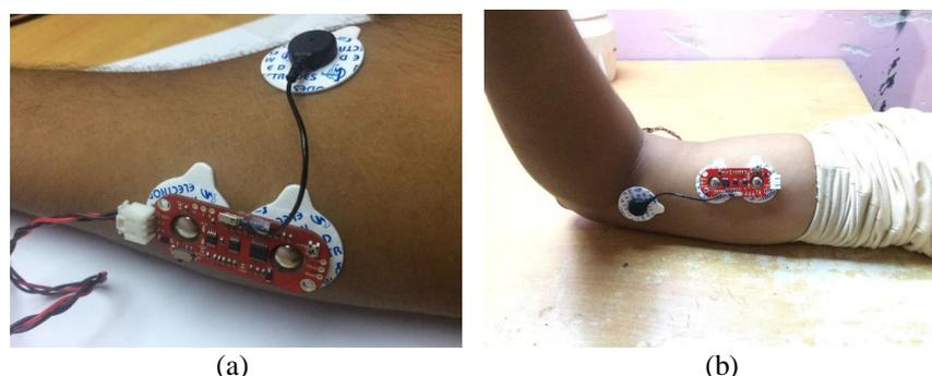
Figure 10: EMG sensor fixed using biomedical electrode pads on (a) the forearm and (b) the biceps.
