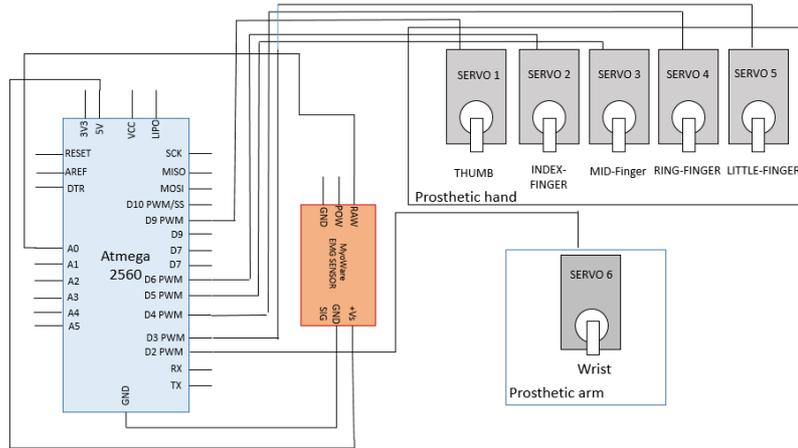
**Figure 6:** Control circuit for prosthetic hand-arm system using EMG sensor.
