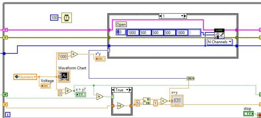
**Figure 8:** LabVIEW block diagram for EMG sensor control scheme.
