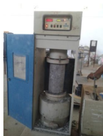
Figure 7 Split tensile test
