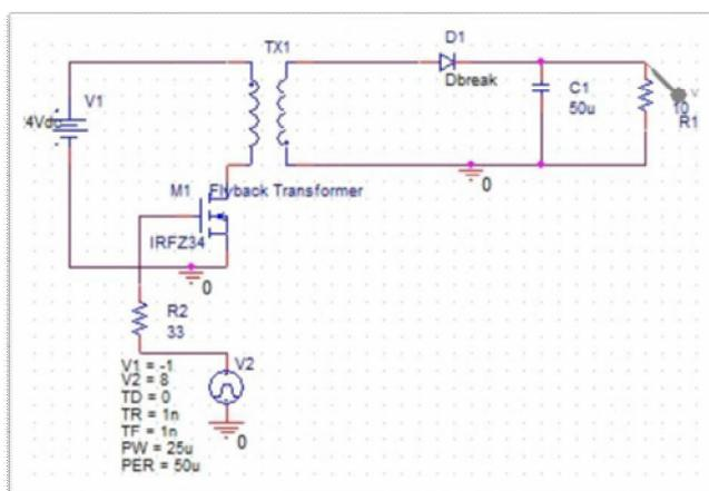
**Figure 1** Circuit diagram of Flyback converter
