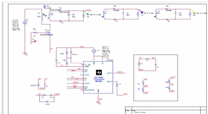
**FIGURE3** CLOSE LOOP SIMULATION WITH UC 1846
