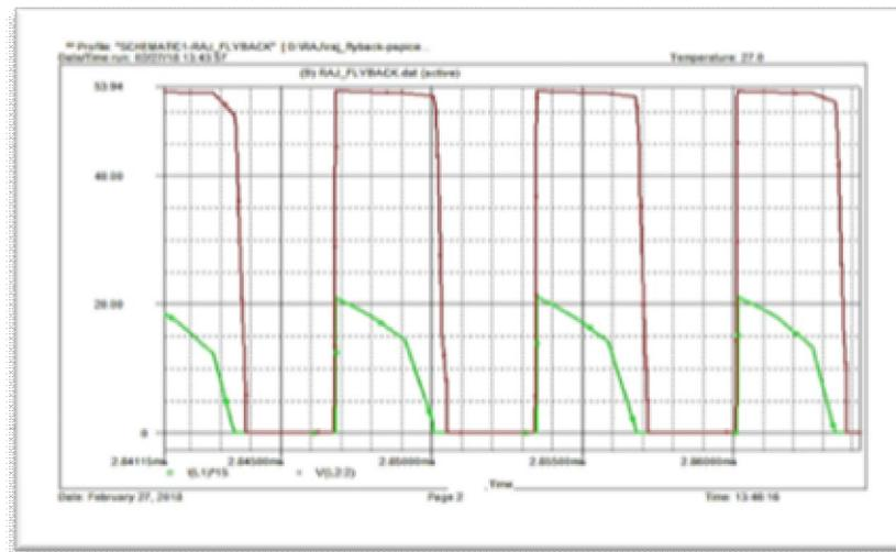
**FIGURE5** INDUCTOR CURRENT AND DUTY CYCLE WAVEFORM
