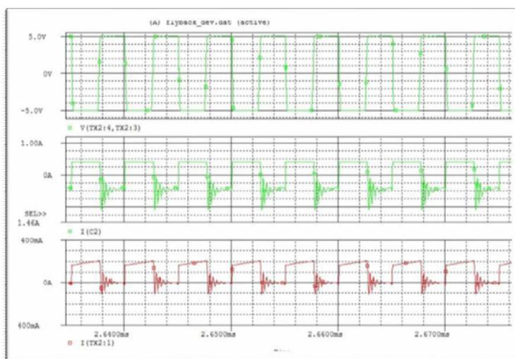
**Figure2** Output results of Flyback converter
