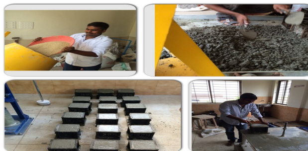
Figure 1: Casting of cubes for Compressive strength
