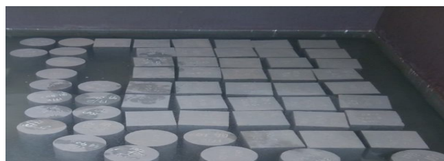
Figure 2: Curing of cubes
