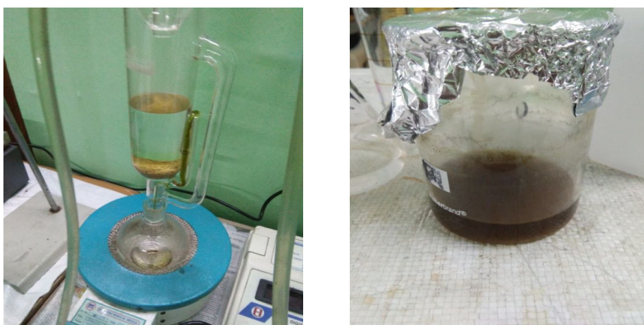
Fig 4 Ethanolic extraction through soxhlet apparatus
