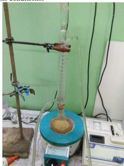
Fig 6 Acidic hydrolysis of Saponin extract to yield diosgenin
