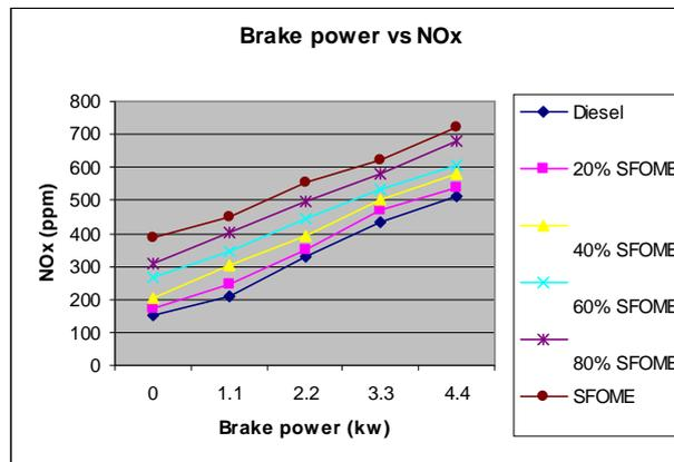
Figure 6 Nitrogen oxides Vs Brake power
