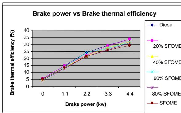
**Figure 3** Brake thermal efficiency Vs Brake power
