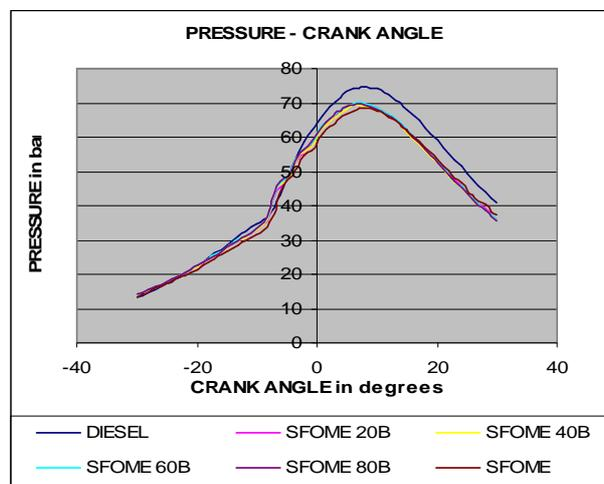
**Figure 11** Pressure – crank angle diagram for SFOME and its blends at full load
