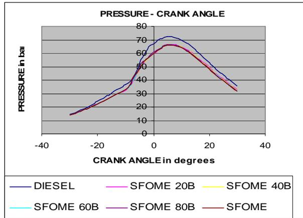
**Figure 10** Pressure – crank angle diagram for SFOME and its blends at 75% load
