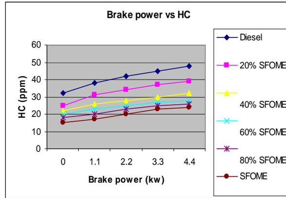
Figure 5 HC Vs Brake power
