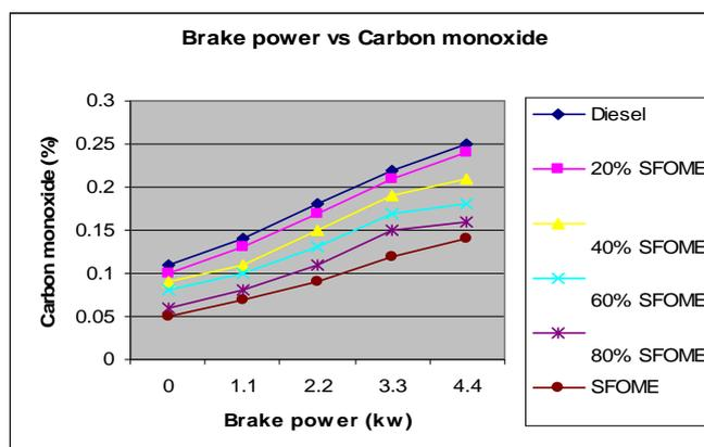
**Figure 4** CO Vs Brake power
