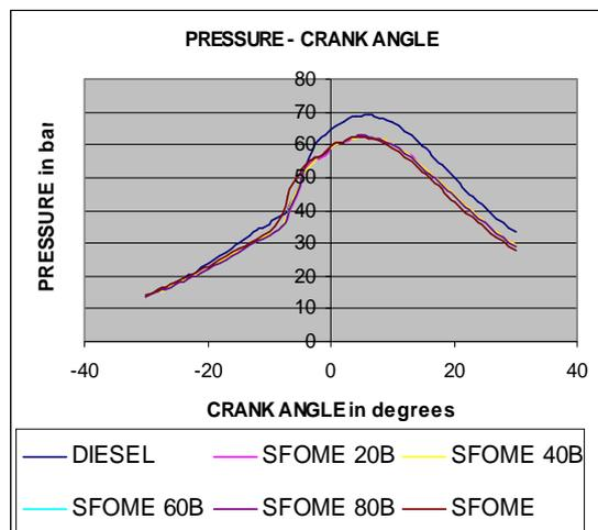
**Figure 9** Pressure – crank angle diagram for SFOME and its blends at 50% load
