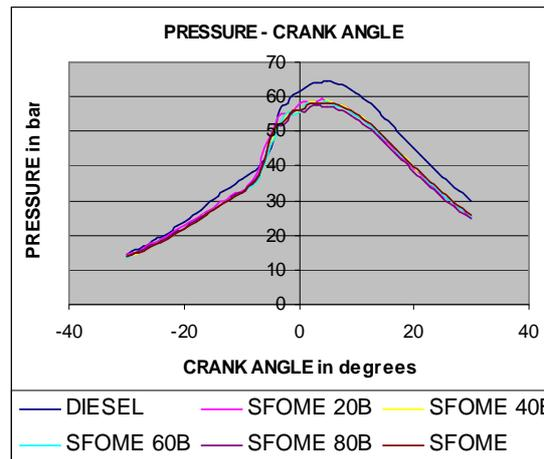
**Figure 8** Pressure – crank angle diagram for SFOME and its blends at 25% load
