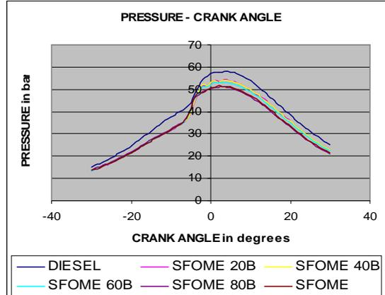
**Figure 7** Pressure – crank angle diagram for SFOME and its blends at no load
