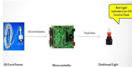
**Figure 8:** Hardware implementation of oil level monitoring system
