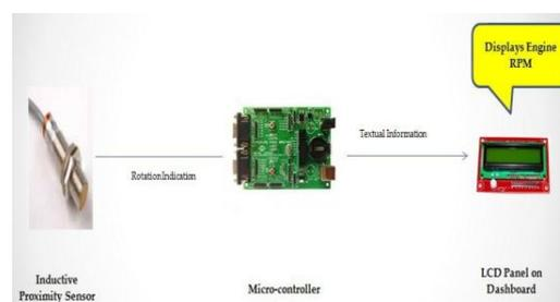
**Figure 2:** Hardware implementation of RPM monitoring System
