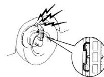
**Figure 11:** Sensor Connection to Brake Pad
