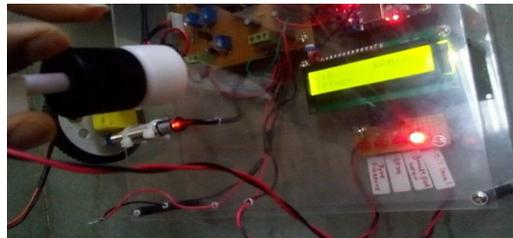
**Figure 9:** Result with warning of visual indication when oil level is low
