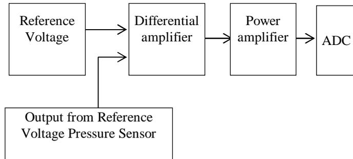
**Figure 4:** Block diagram to measure tyre pressure
