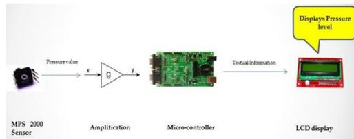
**Figure 5:** hardware implementation of tyre pressure monitoring system
