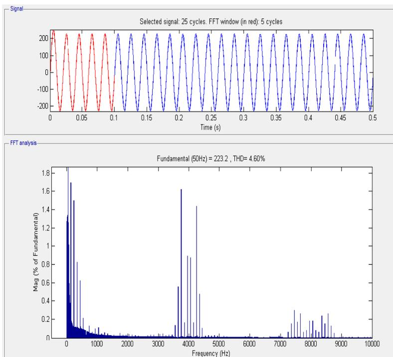
**Figure.10** Output voltage and THD value of open loop model of proposed five level MLI with capacitor filter
