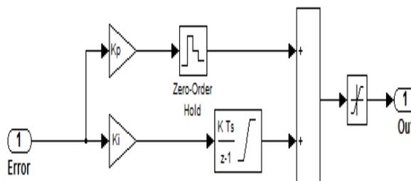
**Figure.3** Simulink diagram of PI controller
