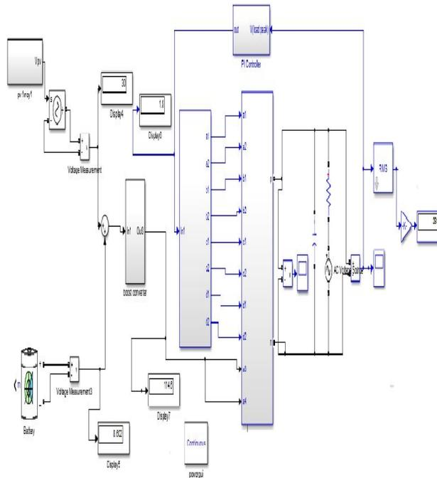
**Figure.11** Simulink diagram of closed loop model of proposed five level MLI with PI controller
