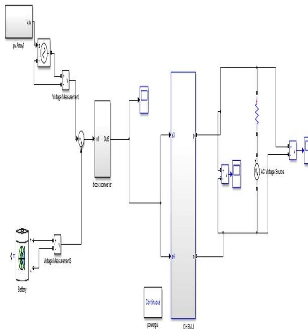
**Figure.8** Simulink diagram of open loop model of proposed five level MLI
