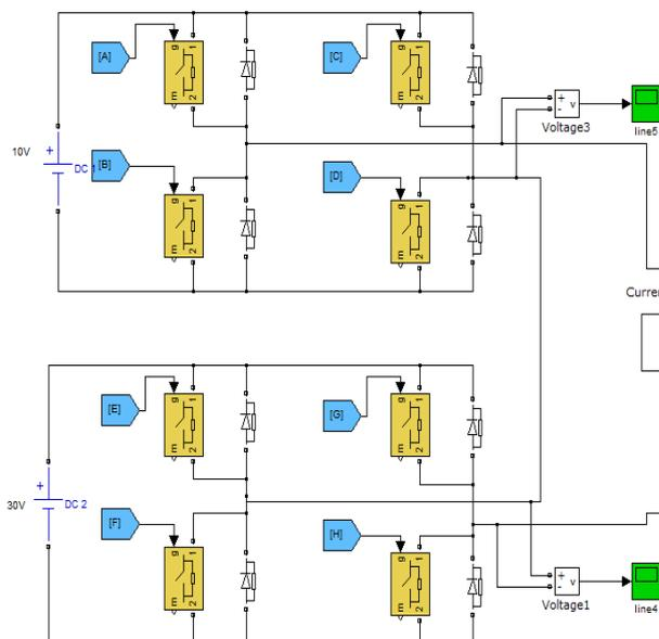
**Figure.6** Simulink diagram of proposed five level MLI
