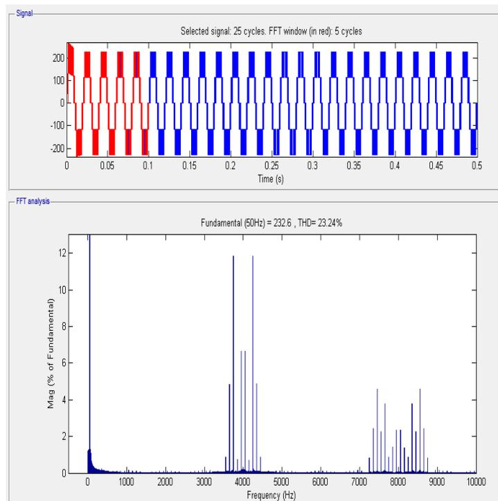
**Figure.9** Output voltage and THD value of open loop model of proposed five level MLI
