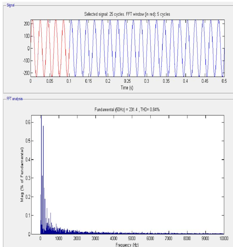
**Figure.12** Output voltage and THD value of closed loop model of proposed five level MLI with PI controller and capacitor filter
