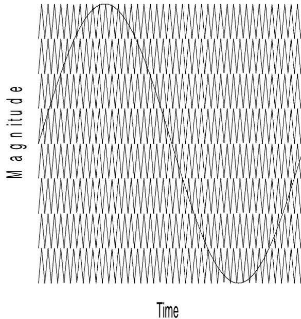
**Figure.2** Multi Carrier-PWM technique
