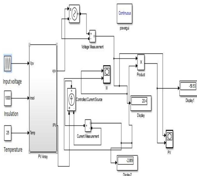
**Figure.5** Simulink diagram of Solar PV cell
