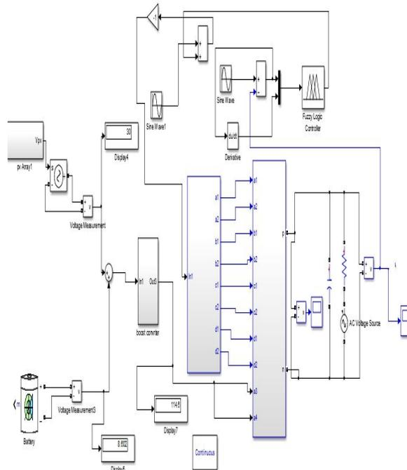
**Figure.13** Simulink diagram of closed loop model of proposed five level MLI with fuzzy controller
