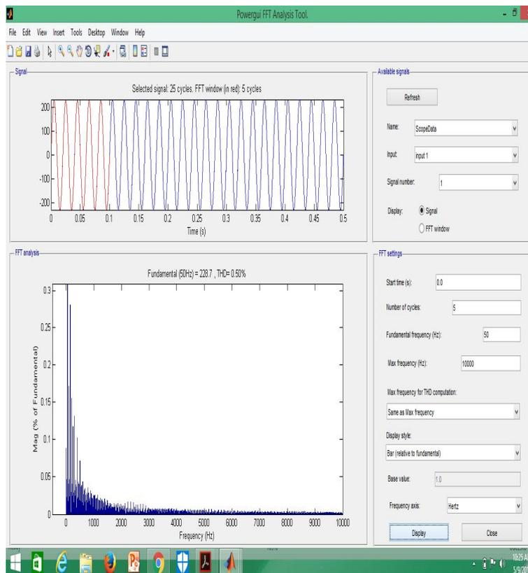
**Figure.14** Output voltage and THD value of closed loop model of proposed five level MLI with fuzzy controller and capacitor filter
