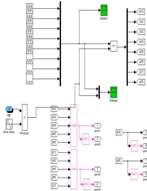
**Figure.7** Simulink diagram of MC-PWM generation for proposed MLI
