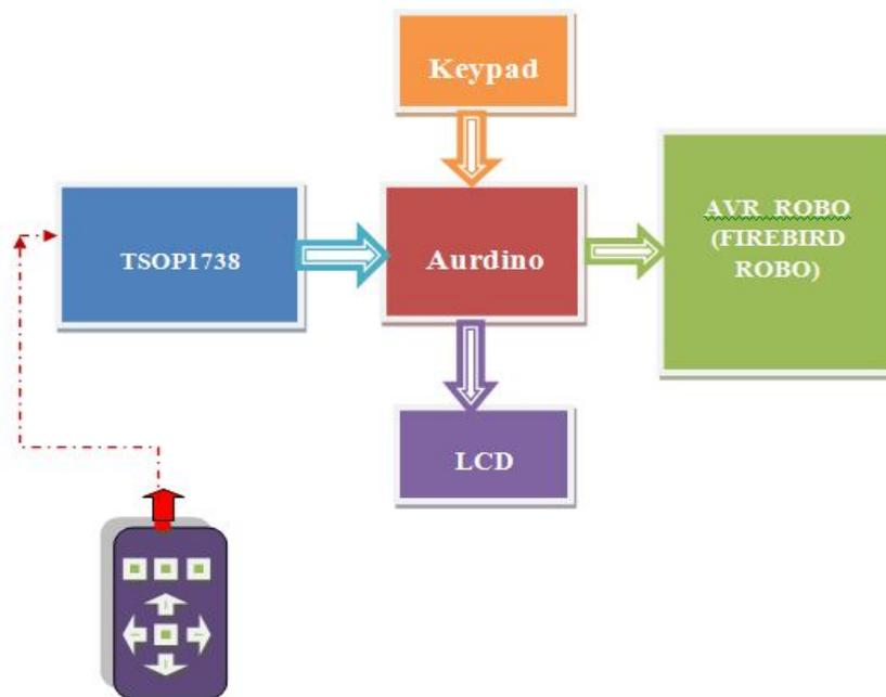
**Figure 2** Waiter Robot Block Diagram
