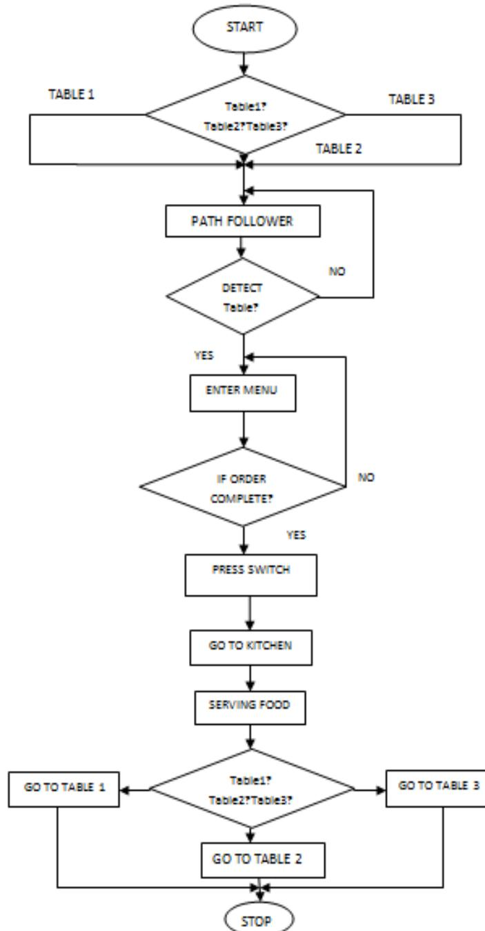
Robot waiter will work on the phenomenon of Line following. Block diagram as shown in figure2, explain our proposed work. we have used three white line sensors and are used for line following and set the waiter robot on line, other two sharp sensors installed on sides are used for table detection. Once the robot is set on the line, now we need to give the command to waiter robot to do the work.
