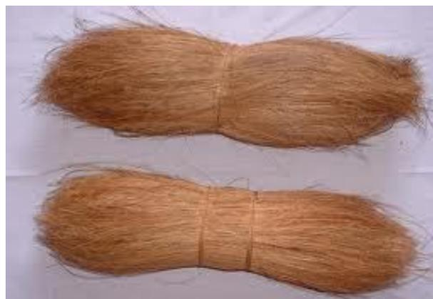
**Figure.1** Jute Fiber (D = 2mm, L = 30 mm)
