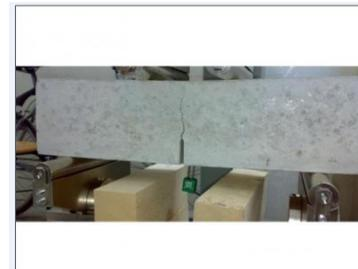
**Figure 6** Flexural Strength Test
