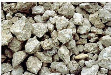
**Figure 2** Recycled Aggregate
