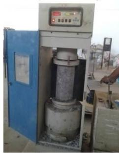
**Figure.5** Split Tensile Test
