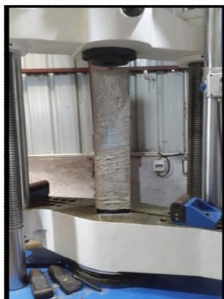
**Figure 1** Column placed in UTM
