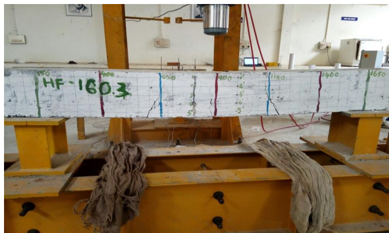
Figure 19 After load removal beam regain its normal position
