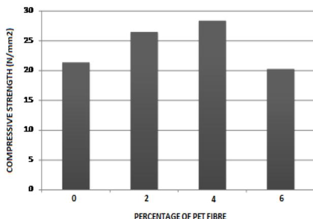
**Figure 3** Compressive Strength Results
