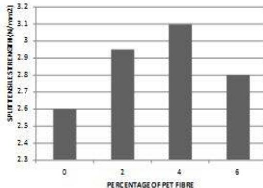
**Figure 4.** Split Tensile Strength Results
