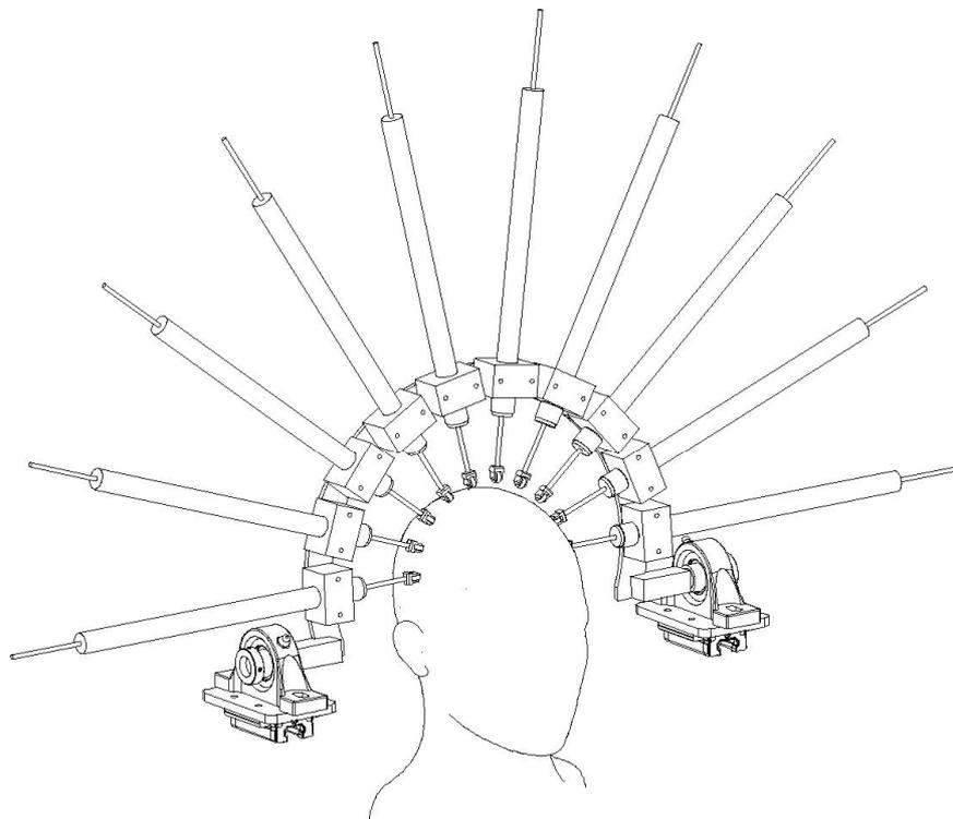
**Fig.3** Arrangement of the object to be scanned and the sensing system.
