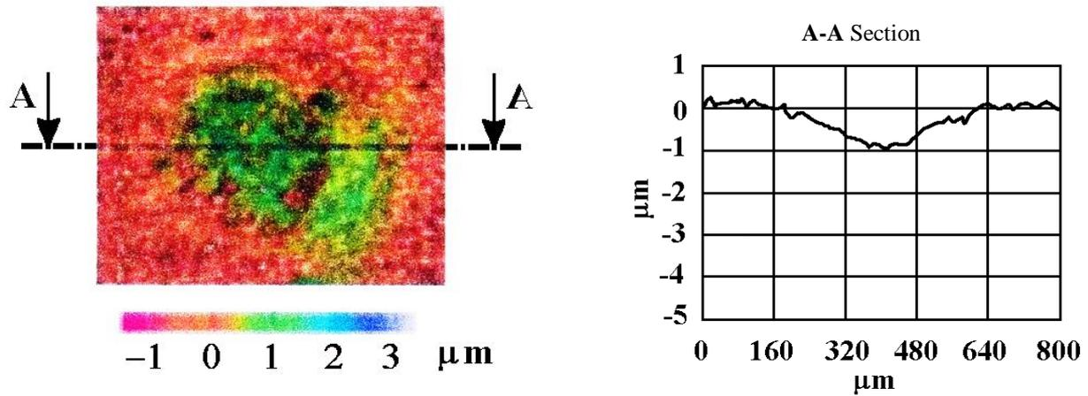
$10^6$  impacts at 800 N impact force; impact duration: 0.3 ms; scar depth:  $\approx 0.7 \mu\text{m}$
