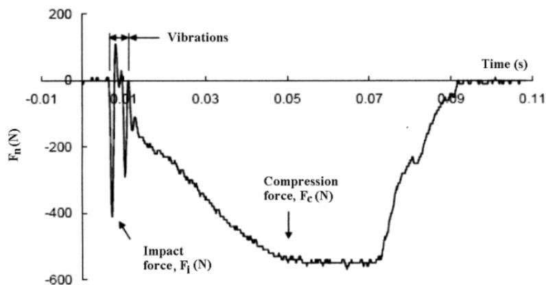
**Figure 6** Time dependence of the impact force with sliding curve, for a cycle  $F_i / F_c = 40 \text{ N} / 34.64 \text{ N}$
