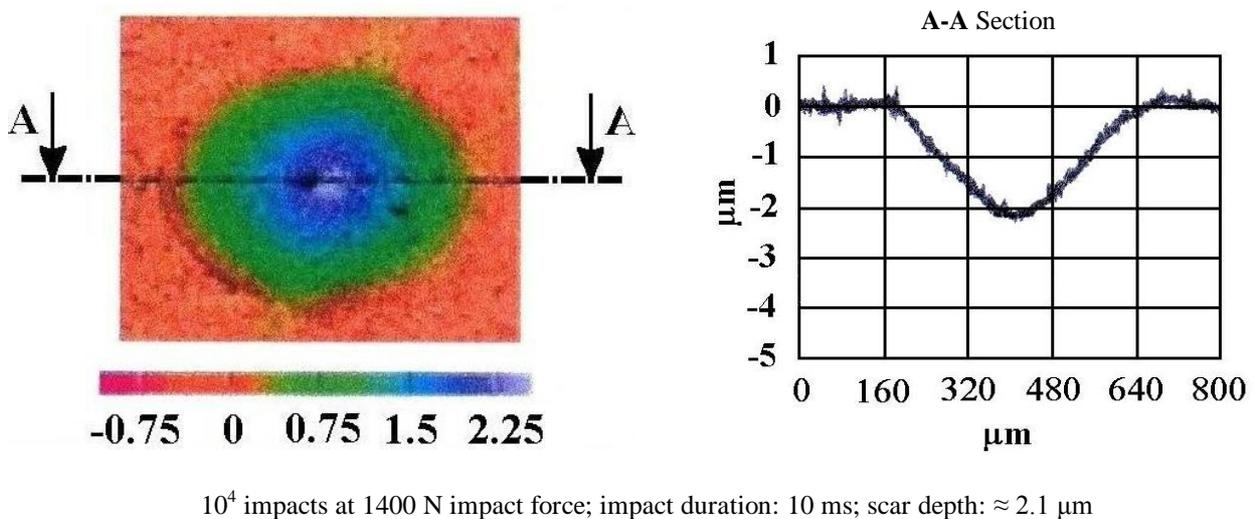
**Figure 3** Depths of remaining scars on TiN / SS316L at 1400 N. determined by measurements of confocal 3D microscopy (left) and profilometry (right), depending on the duration of the impact
