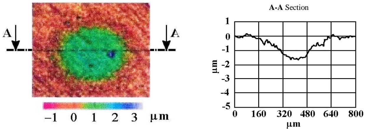
$10^6$  impacts at 900 N impact force; impact duration: 0.3 ms; scar depth:  $\approx 0.85 \mu\text{m}$
