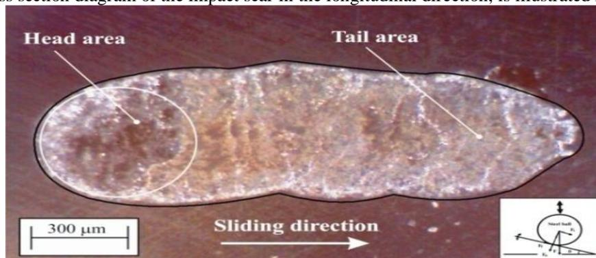
**Figure 7** Microfotography of cyclic impact with sliding scar after 10000 inclined impacts at  $30^\circ$
