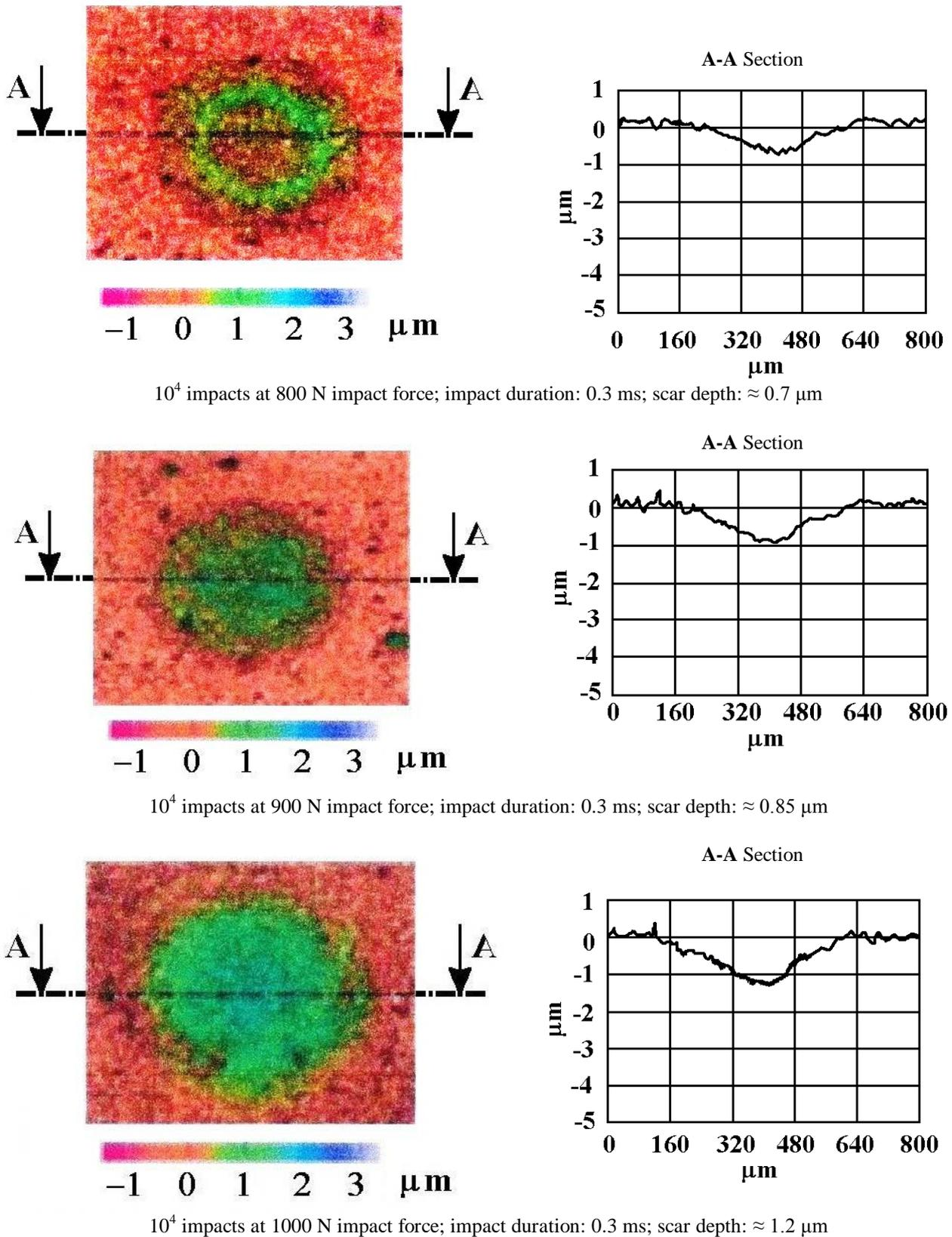
**Figure 4** Depths of remaining scars on TiN/SS316L at 800 N, determined by measurements of 3D confocal microscopy (left) and profilometry (right), at  $10^4$  impacts of 0.3 ms, depending on the size of the impact force
