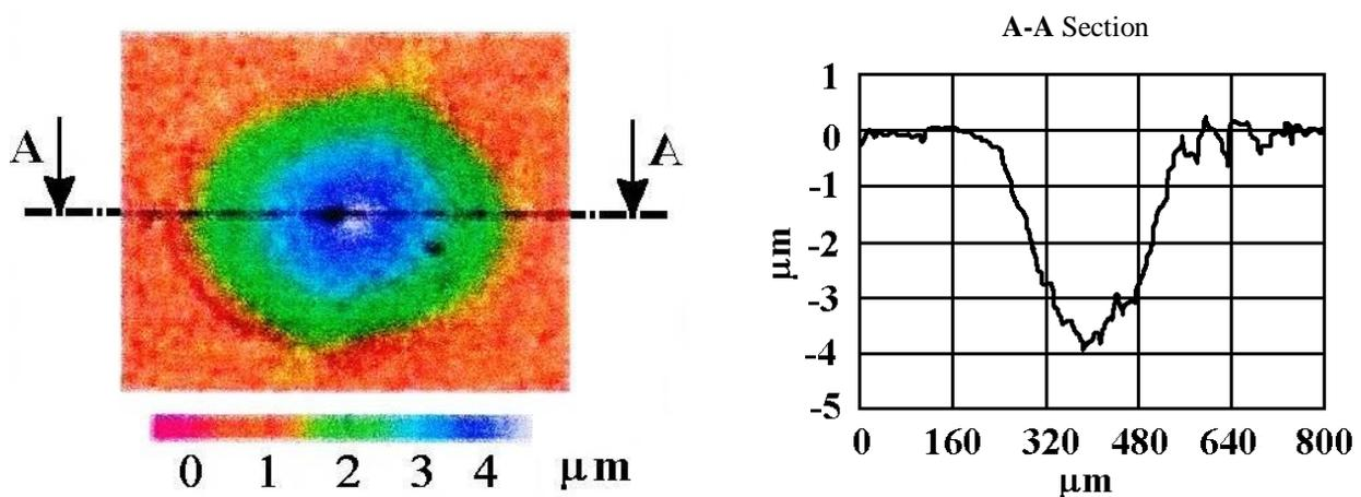
$10^6$  impacts at 1000 N impact force; impact duration: 0.3 ms; scar depth:  $\approx 1.2 \mu\text{m}$
