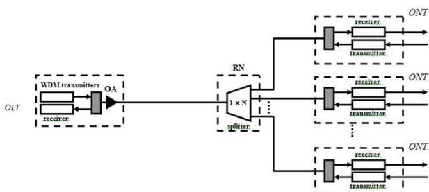
**Figure 4** The general LR-PON network architecture
