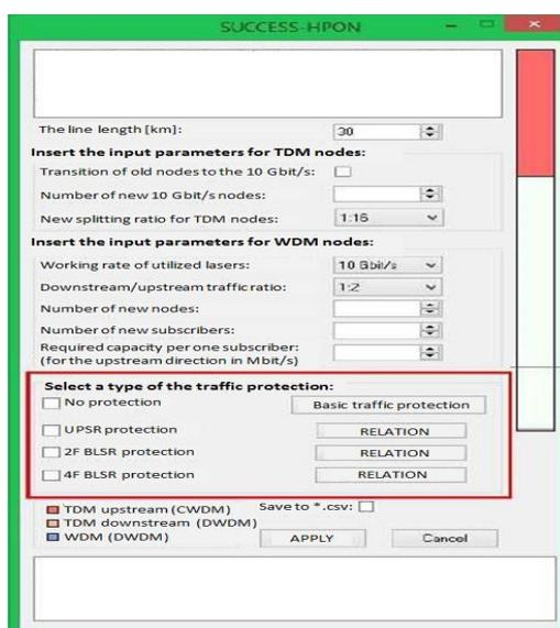
**Figure 7** The SUCCESS HPON configuration window with extended traffic protections
