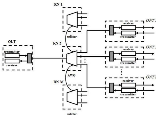
**Figure 1** The general WDM/TDM-PON network architecture
