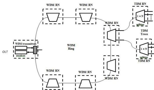
**Figure 3** The general SARDANA HPON network architecture
