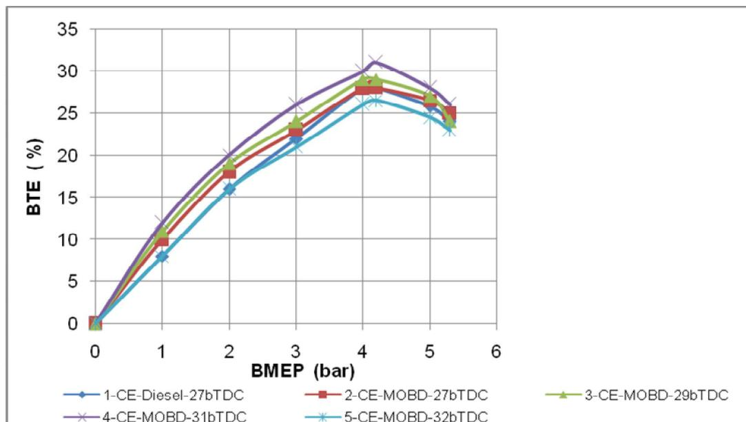
**Fig. 3** Variation of brake thermal efficiency (BTE) with brake mean effective pressure (BMEP) in conventional engine (CE) with biodiesel at various injection timings at an injector opening pressure of 190 bar.
