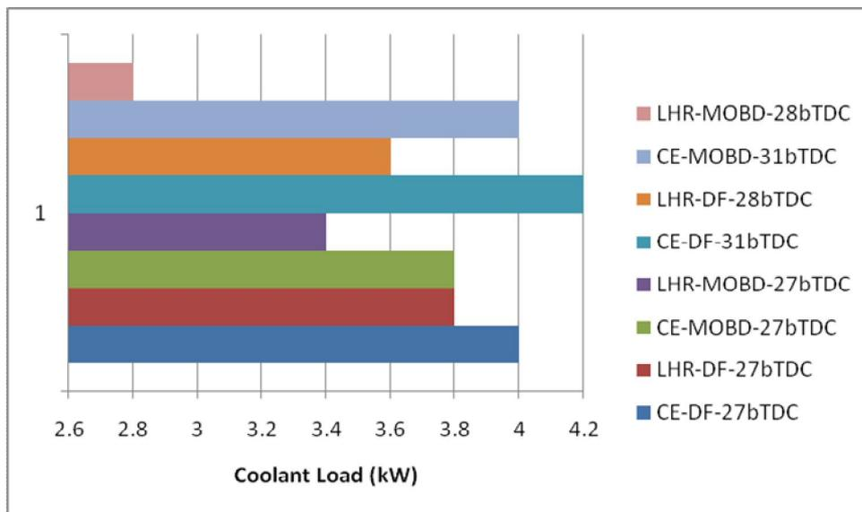
**Fig.9.** Bar charts showing variation of coolant load at full load with mahua oil biodiesel (MOBD)
