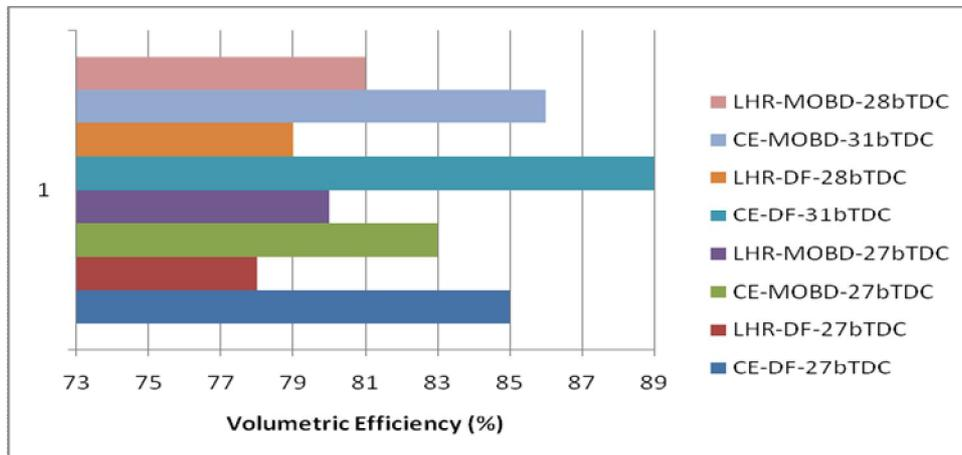
Fig.8.Bar charts showing variation of volumetric efficiency at full load with mahua oil biodiesel (mobd)
