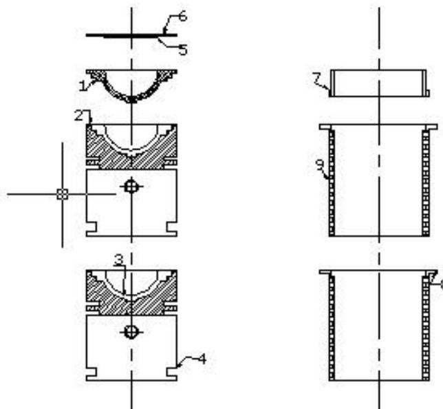
**Fig.1** Assembly details of air gap insulated piston, air gap insulated liner and ceramic coated cylinder head
