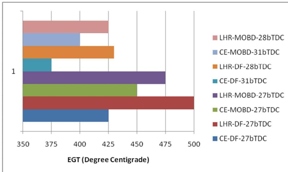
**Fig.7.** Bar charts showing variation of exhaust gas temperature (egt) at full load with mahua oil biodiesel (mobd)
