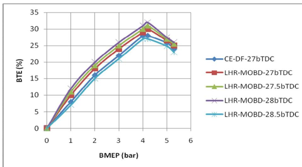
**Fig.4.** Variation of brake thermal efficiency (BTE) with brake mean effective pressure (BMEP) in engine with LHR combustion chamber with biodiesel at various injection timings at an injector opening pressure of 190 bar.
