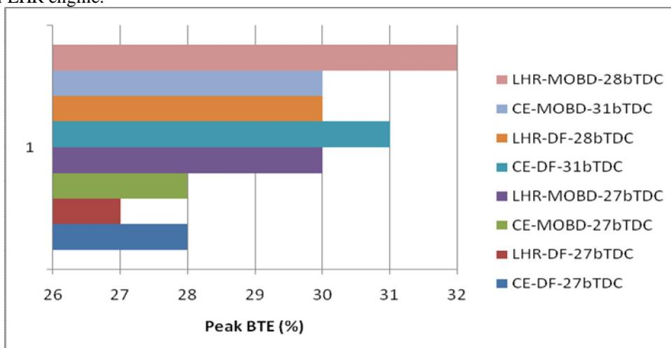
**Fig.5.** Bar charts showing the variation of peak brake thermal efficiency (BTE) with mahua oil biodiesel
