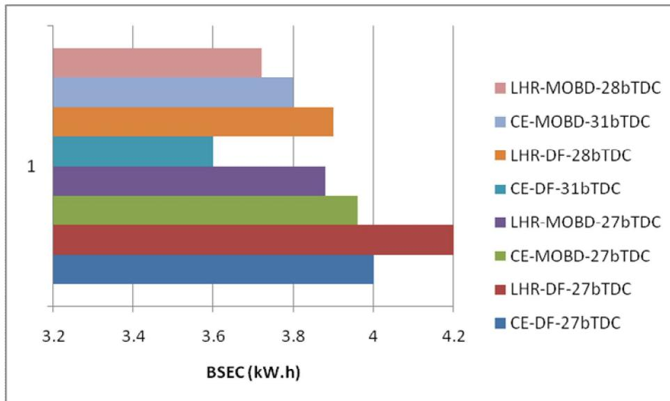
**Fig.6.** Bar charts showing the variation of brake specific energy consumption (BSEC) at full load with biodiesel operation (MOBD)
