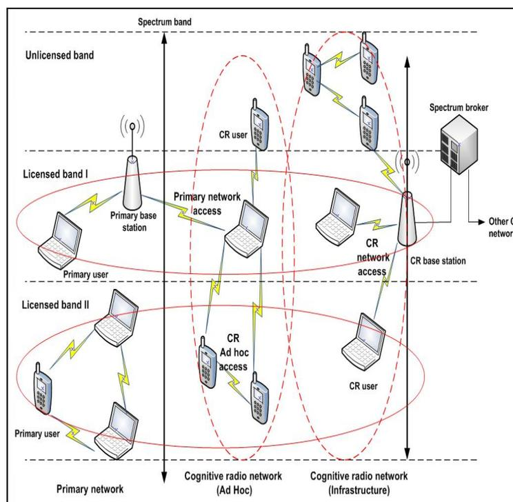
**Figure 3** The cognitive radio network architecture [8]
