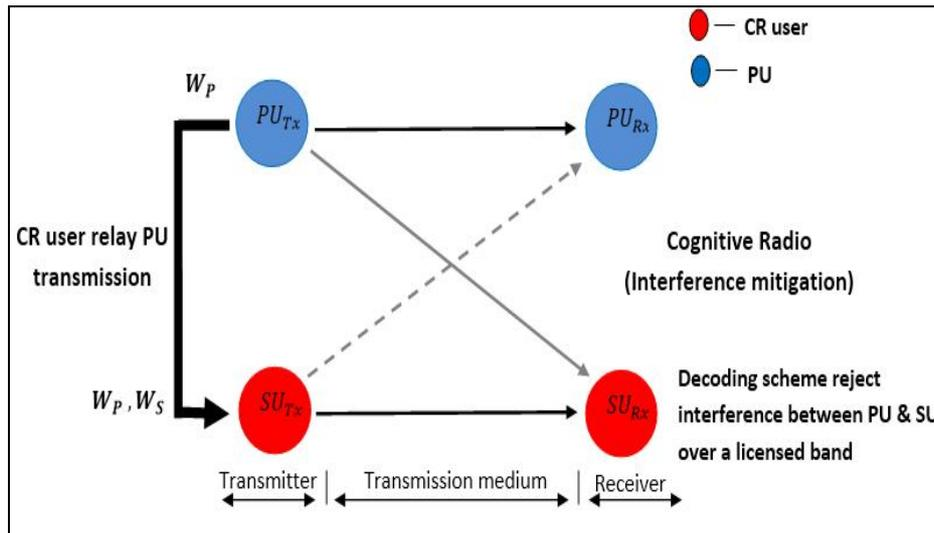
**Figure 7** The overlay spectrum sharing over the interference channel model [24]
