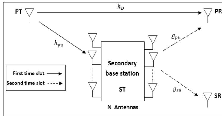
**Figure 9** System model of cooperation relay in overlay spectrum sharing technique [26]
