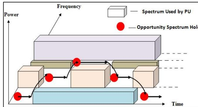
**Figure 1** The Dynamic spectrum access technique
