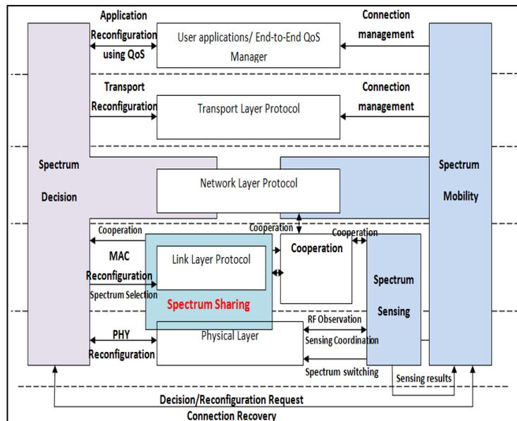
**Figure 4** CR capabilities at the CRN protocol stack [7]
