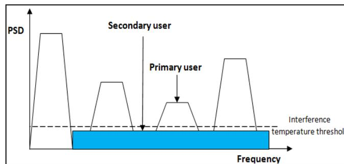
**Figure 6** The underlay spectrum sharing [1]
