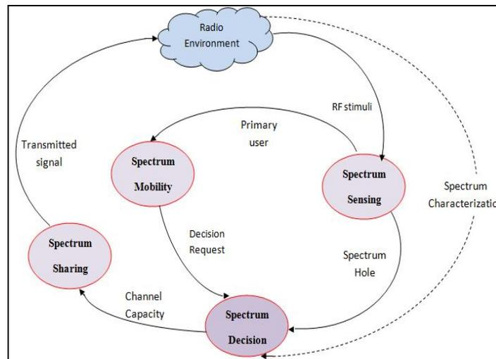
**Figure 2** The cognitive radio cycles [7]
