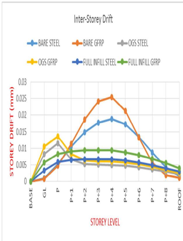
Figure 6. Storey Drift at each storey for P+9 model
