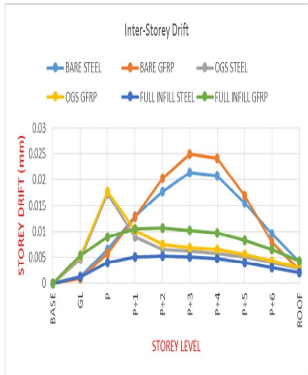
**Figure 5.** Storey Drift at each storey for P+7 model
