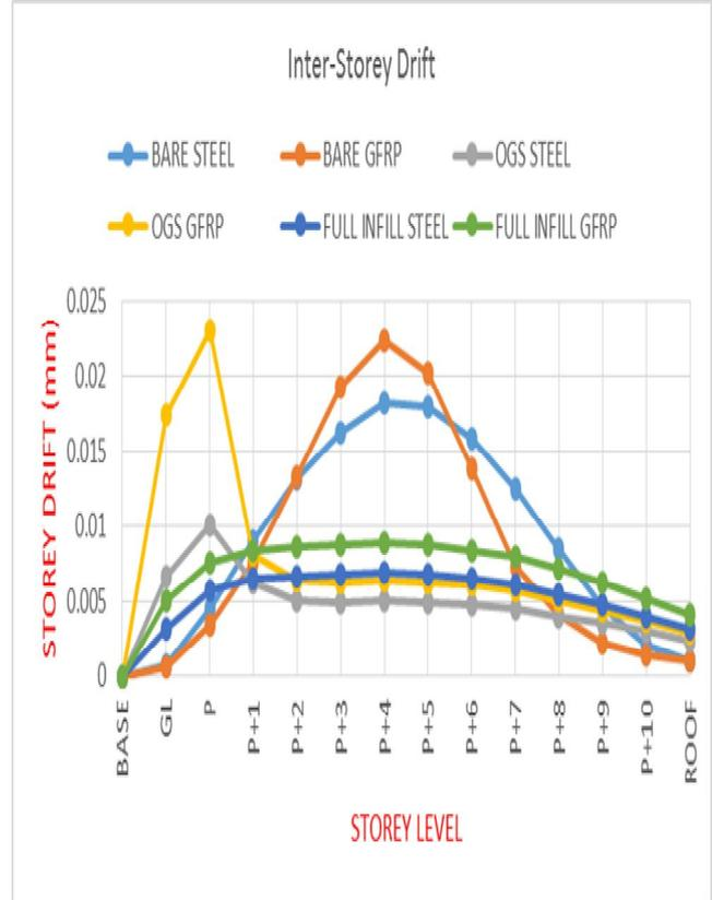
Figure 7. Storey Drift at each storey for P+11 model
