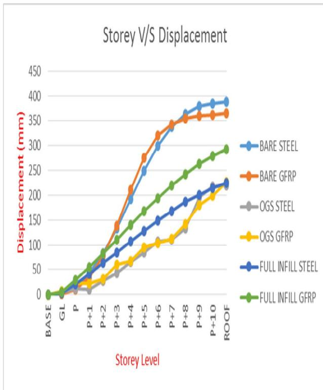
**Figure 4.** Max. Displacement at each storey for P+11 model
