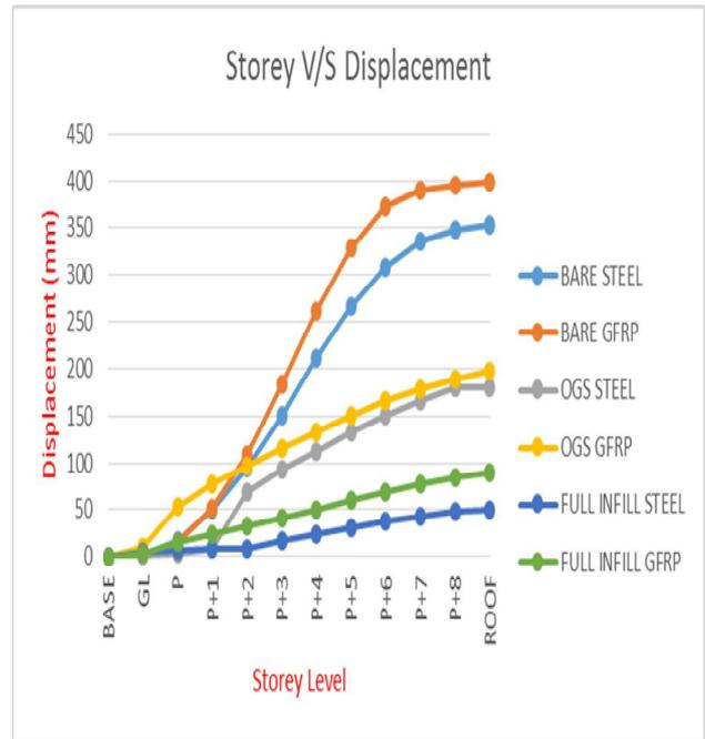
**Figure 3.** Max. Displacement at each storey for P+9 model
