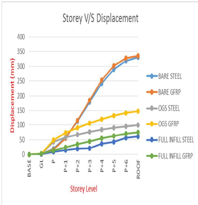
**Figure 2.** Max. Displacement at each storey for P+7 model model
