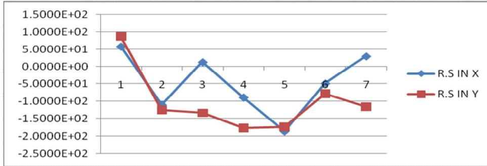
**Figure 6:** RESIDUAL STRESS PROFILES WITH FOUR DIFFERENT CUTTING FLUIDS.
