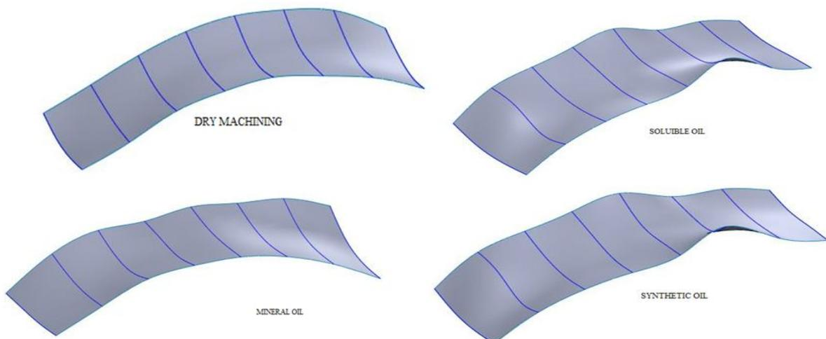
**Figure 8:** PROFILES OF THE WORK PICES AFTER MACHINING WITH DIFFERENT CUTTING FLUIDS
