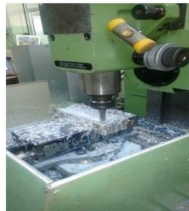
**Figure 2:** DECKEL FP4A CNC machine
