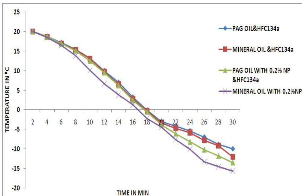
We kept the refrigerating space under observation for 30 minutes. Meanwhile we have also taken readings of temperature of the refrigerating space in every two minutes interval and found out that the temperature has reduced from 20°C to -10°C, -12°C, -13.5°C & -15.6°C for the mixture of PAG Oil and R134a, Mineral Oil and R134a, PAG Oil with 0.2% mass fraction of nanoparticles and R134a, Mineral Oil with 0.2% mass fraction of nanoparticles and R134a respectively.
