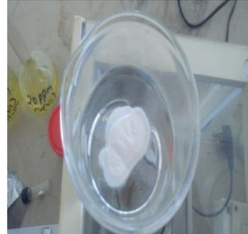
**Fig.2:** nanoparticles added to PAG Oil
