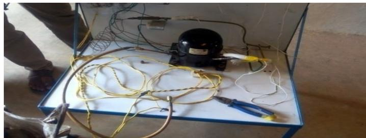
**Fig.3:** Release of Air if present in the system
