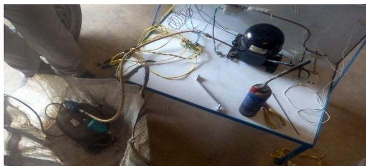
**Fig.4 :** Vacuum Pump is attached to the service Port for evacuation
