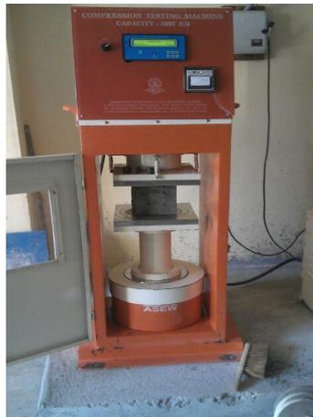
**Fig-1** Cube Compression Test
