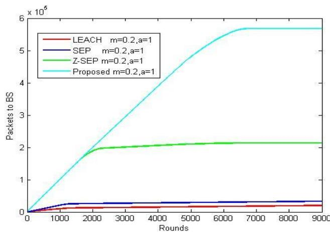
**Fig. 6:** Packets send to BS versus Rounds
