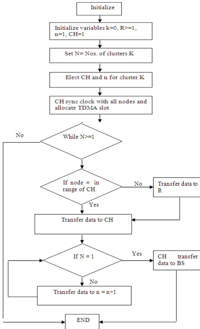
**Fig. 1:** Flow Chart for Data Transmission in CRS Approach
