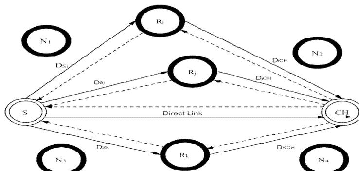
**Fig. 2:** Source Node Communicate with CH directly or via Relay Nodes [16]
