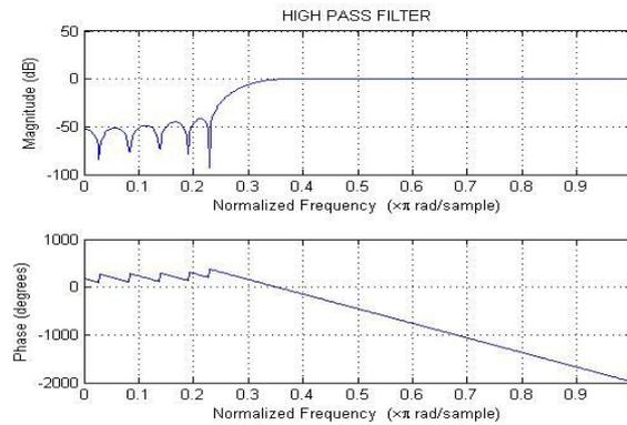
Fig 3: High pass filter
