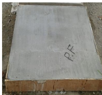
Figure. 12 Mortar Placing Above The Palm Fibre
