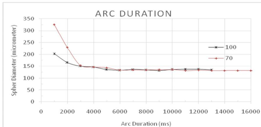
**Figure 2** Duration calibration curves at two different arc voltages
