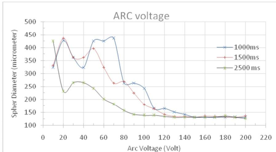
**Figure 1** Voltage calibration curves at three different arc durations
