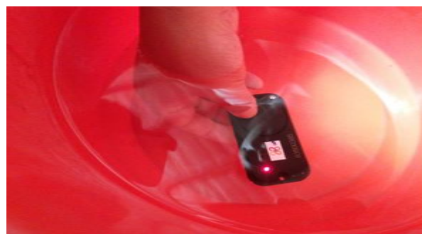
Figure3: Tag immersed in water
