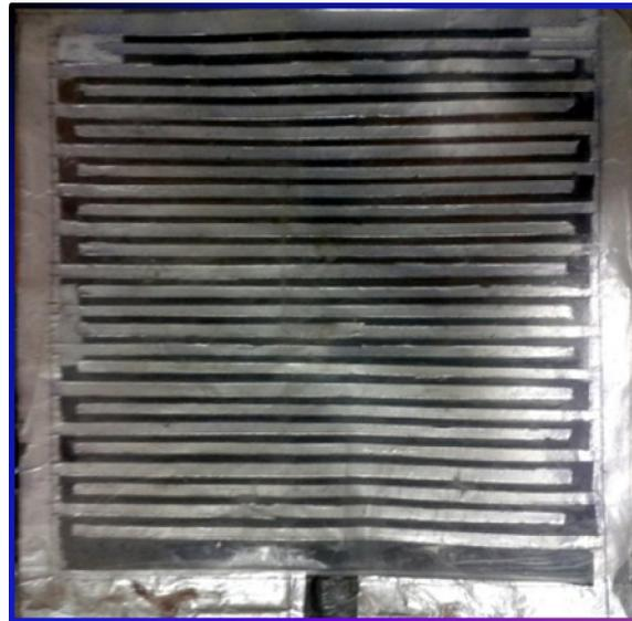
**Figure 4** Flexible electro adhesive pad developed using Aluminum electrodes
