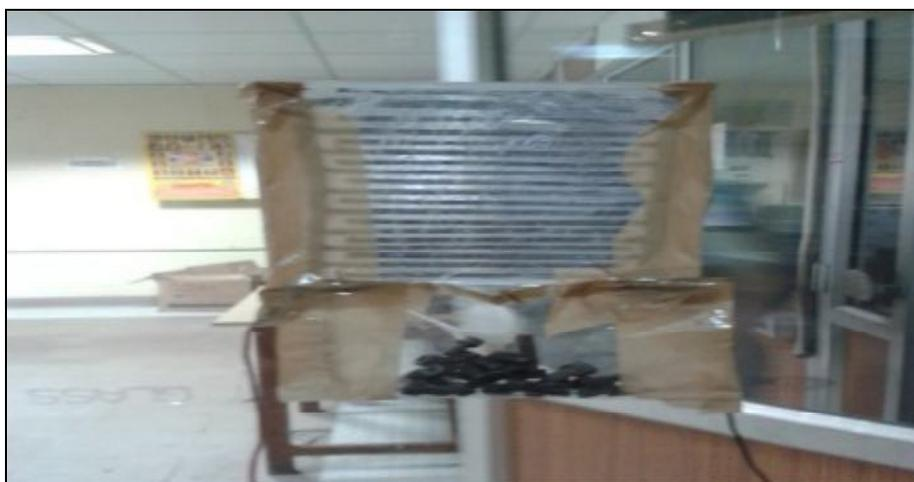
**Figure 5** Application of weights on the different Electro adhesive pads on glass surface
