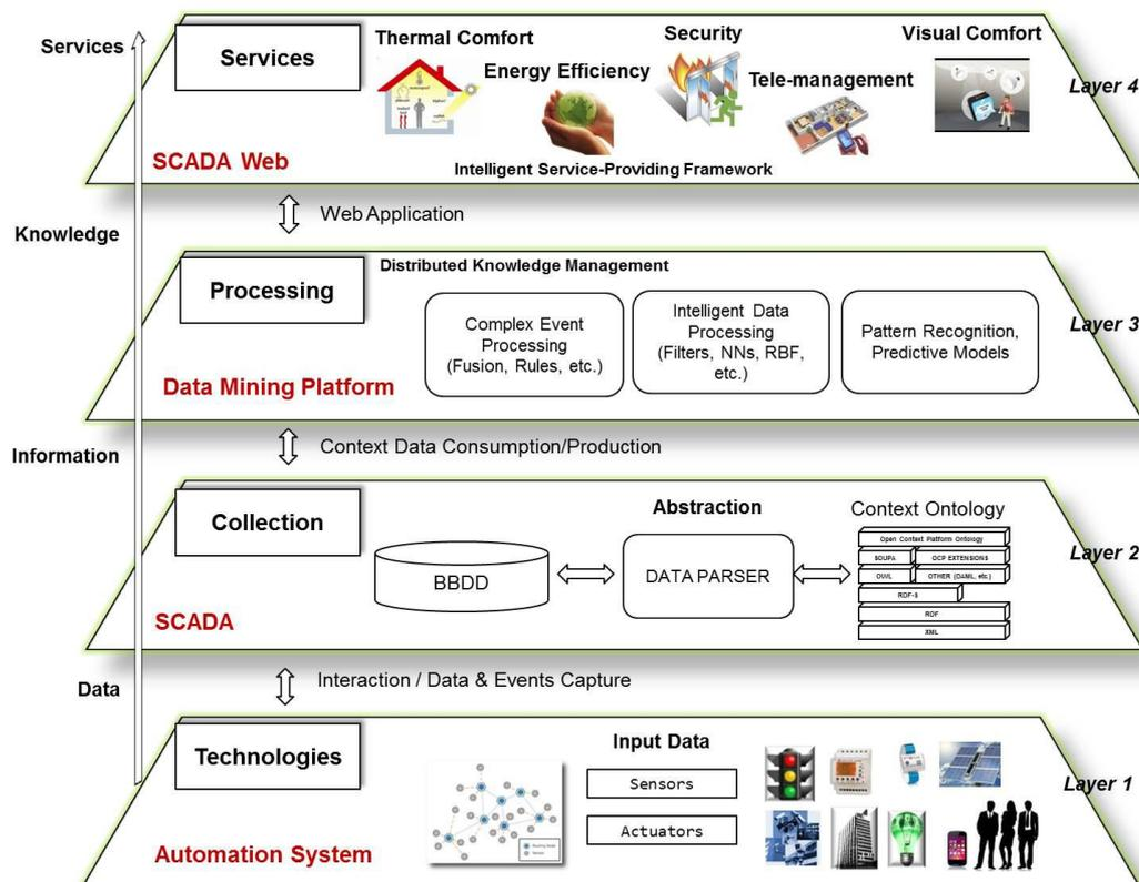
**Figure1** IOT Architecture For Smart Building
