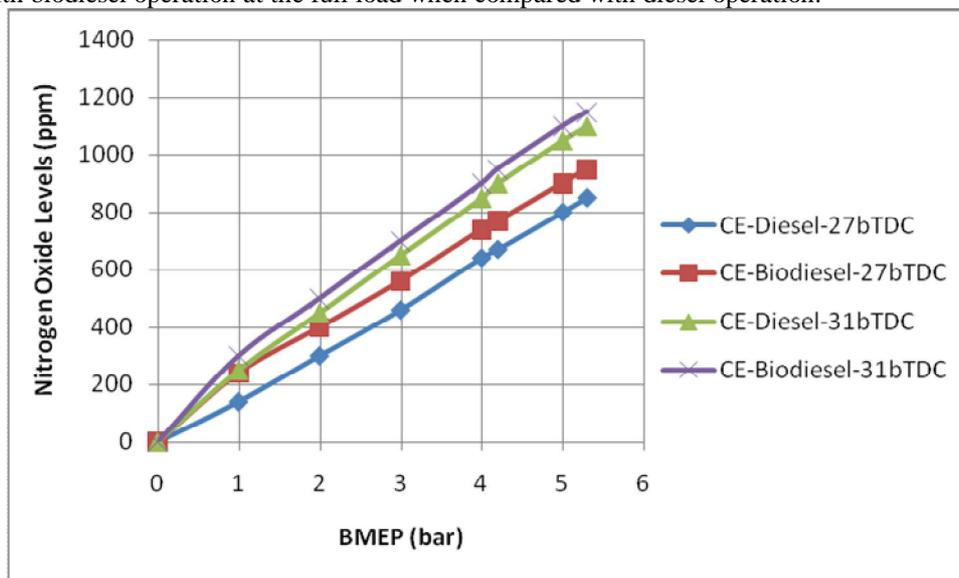
**Fig.8** Variation of nitrogen oxide levels (NO<sub>x</sub>) with brake mean effective pressure with test fuels in conventional engine (CE) at recommended and optimum injection timing.
