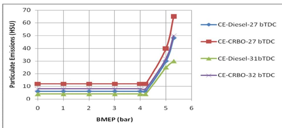
**Fig.4** Variation of particulate emissions with brake mean effective pressure with test fuels in conventional engine (CE) with vegetable oil and diesel at recommended and optimum injection timing
