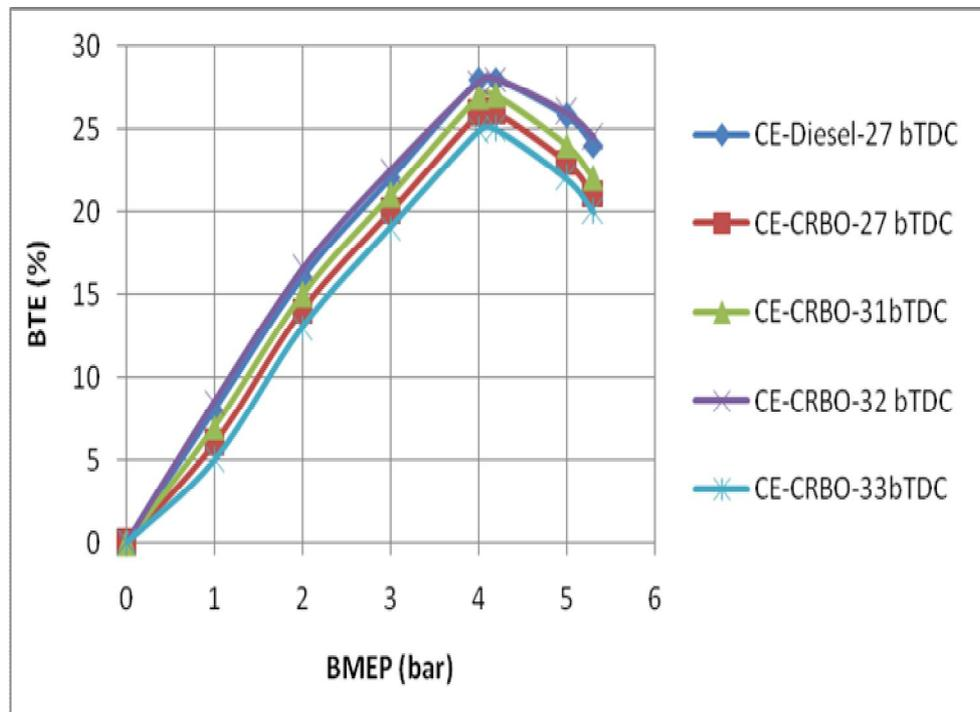
**Fig.2.** Variation of brake thermal efficiency (BTE) with brake mean effective pressure (BMEP) in conventional engine (CE) at different injection timings with crude rice brawn oil (CRBO) operation.
