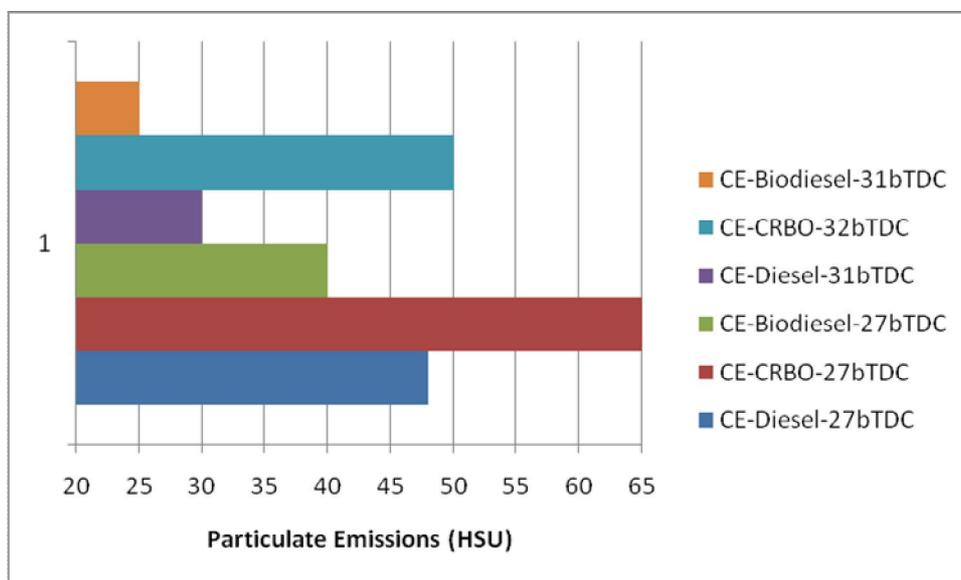
**Fig. 6.** Bar charts showing the variation of particulate emissions in Hartridge smoke unit (HSU) at full load operation with test fuels at recommended and optimized injection timings at an injector opening pressure of 190 bar.
