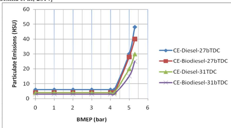
**Fig.5** Variation of particulate emissions with brake mean effective pressure with test fuels in conventional engine (CE) with biodiesel and diesel at recommended and optimum injection timing.
