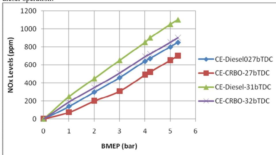
**Fig.7** Variation of nitrogen oxide levels (NO<sub>x</sub>) with brake mean effective pressure with test fuels in conventional engine (CE) with vegetable oil and diesel at recommended and optimum injection timing.
