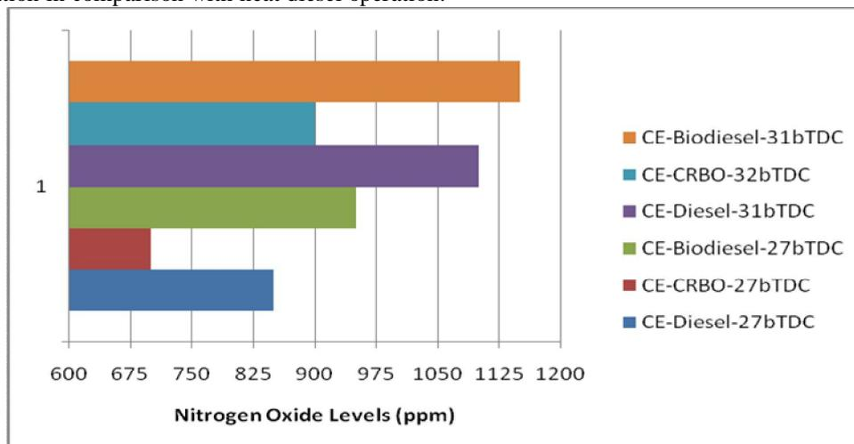
**Fig. 9.** Bar charts showing the variation of nitrogen oxide levels (NO<sub>x</sub>) at full load operation with test fuels at recommended and optimized injection timings at an injector opening pressure of 190 bar.
