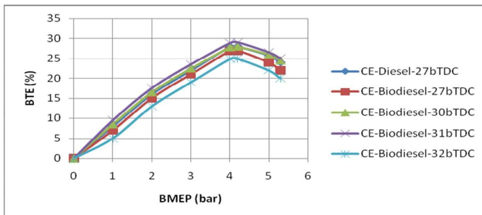
**Fig.3.** Variation of brake thermal efficiency (BTE) with brake mean effective pressure (BMEP) in conventional engine (CE) at different injection timings with rice brawn biodiesel operation.
