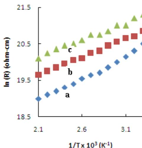
**Fig. 1.** Shows variation of resistivity verses inverse temperature for thickness a)  $t = 0.2530 \mu\text{m}$ , b)  $t = 0.2100 \mu\text{m}$  and c)  $t = 0.1985 \mu\text{m}$
