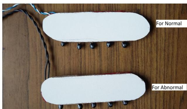
**Fig 1:** Temperature Measuring Probes.
