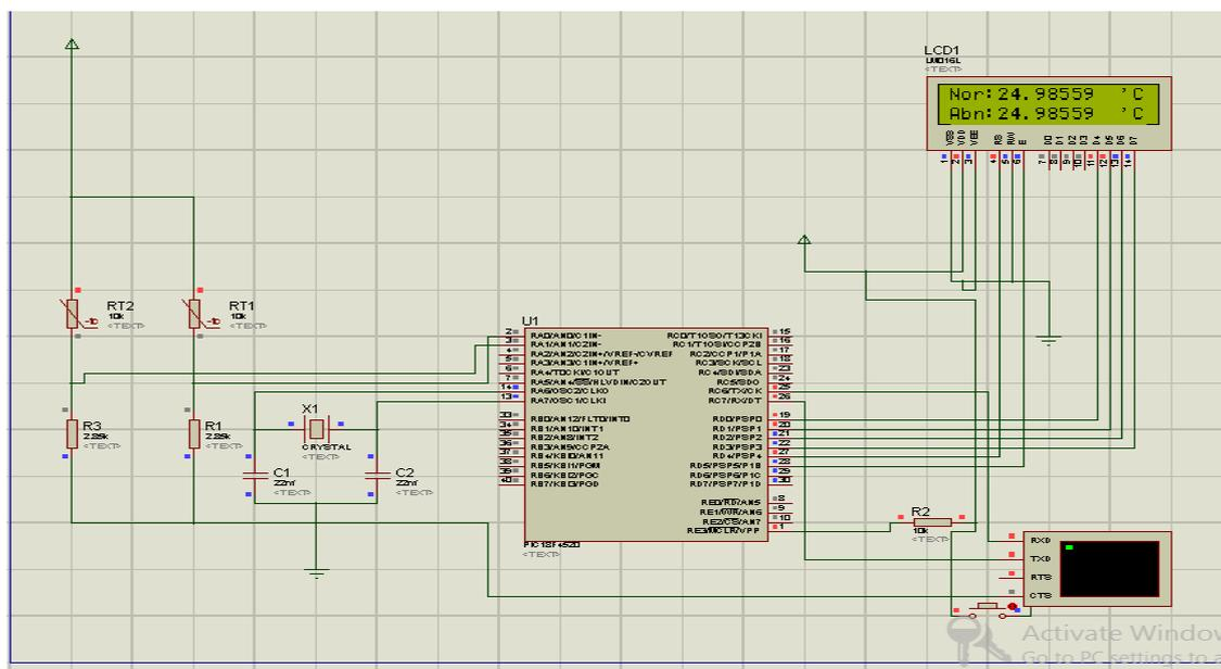
**Fig 3:** Circuit diagram for skin temperature measurement
