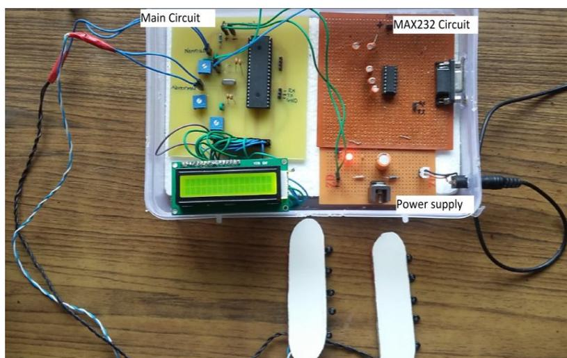
**Fig 5:** Temperature Measuring Module.
