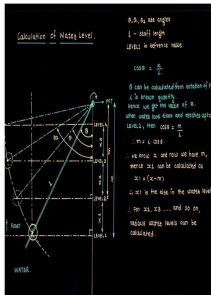
**Figure 2** Concept of level Measurement
