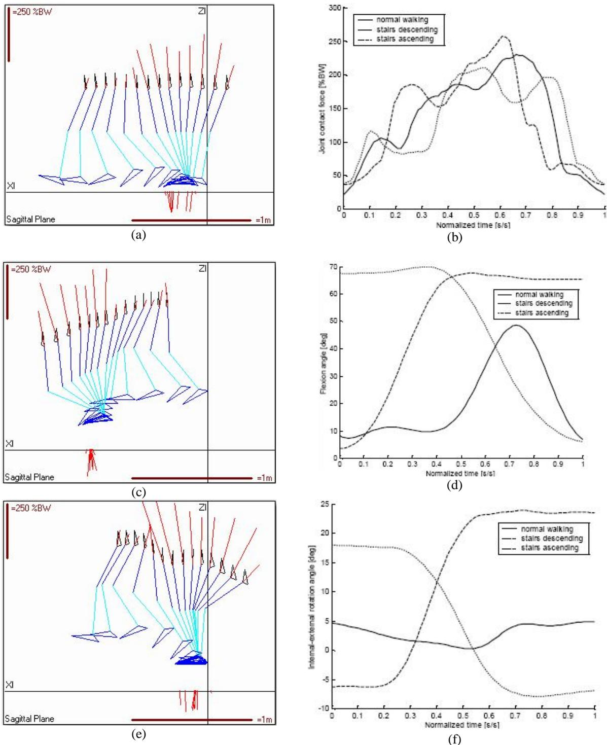
**Figure 2** Dynamic conditions during all activities: kinematics of the lower member from S.J.G. Taylor and P.S. Walker, 2001 [19] (a – normal walking, b – stairs descending, c – stairs ascending) and loading from T. Villa, 2004 [20], and kinematics from S.J.G. Taylor, 2001, of the joint surfaces (d – contact force, e – flexion angle, f – internal-external rotation angle).
