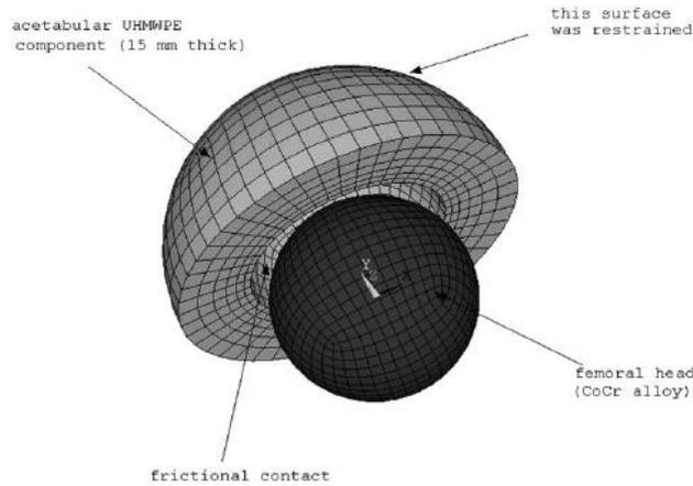
**Figure 1** Finite element model for the hip artificial joint
