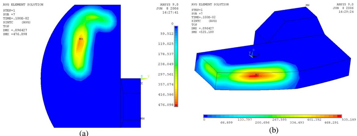
**Figure 8** The damage score map (a) at the contact surface, (b) in the subsurface.
