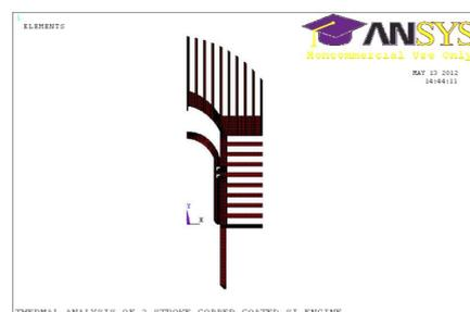
**Figure 3** Mesh employed in the thermal analysis for CCE
