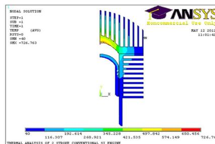
**Figure 4** Isotherms of thermal analysis for CE
