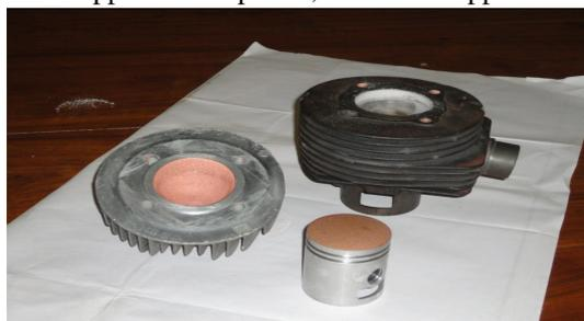
**Plate 1** Photographic view of copper coated piston, liner and copper coated cylinder head
