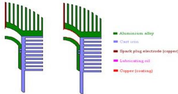
**Figure 1** Configuration of the assembly of piston, liner and cylinder head for CE and CCE
