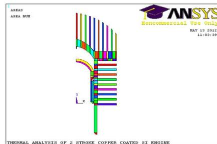
**Figure 2** Geometric model created for the thermal analysis for CCE
