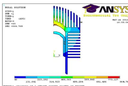
**Figure 5** Isotherms of thermal analysis for CCE
