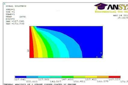
**Figure 7** Isotherms from FEA in the lubricating oil between piston and liner inner surface for CCE
