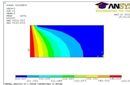
**Figure 6** Isotherms from FEA in the lubricating oil between piston and liner inner surface for CE
